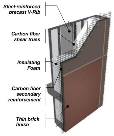
Fig. 1 Lightweight cladding reinforced with carbon fiber
