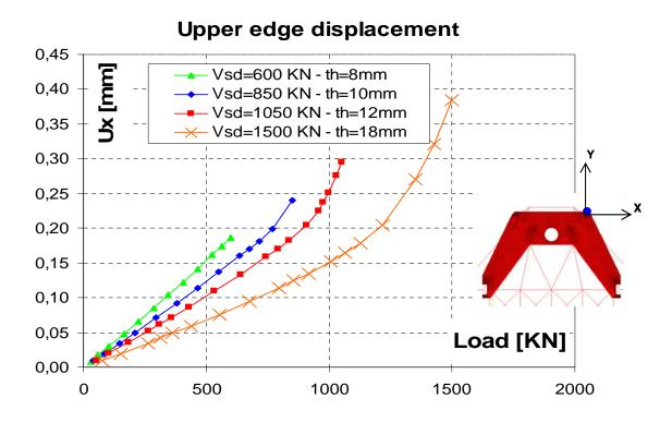
Fig.12: Load-displacement for the external point of the frame, for the symmetric cases.
