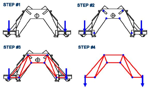
Fig.5: Main aspects of the load path for the cable-stayed innovative connection under study.
