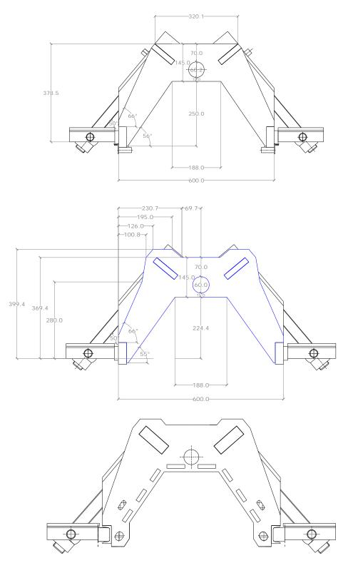
Fig.14: Evolution of the configuration of the cable-stayed bracket as consequences of the development of the analysis.
