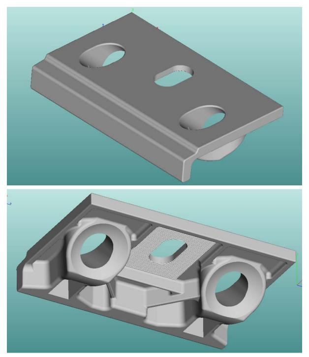
Fig.18: Top and bottom view of the initially proposed configuration of the external bracket.
