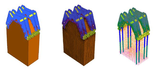
Fig.15: Three-dimensional modeling of the connection and of the segment of concrete columns; on the left, only the steel parts (plates of the frame and longitudinal bars) are represented.
