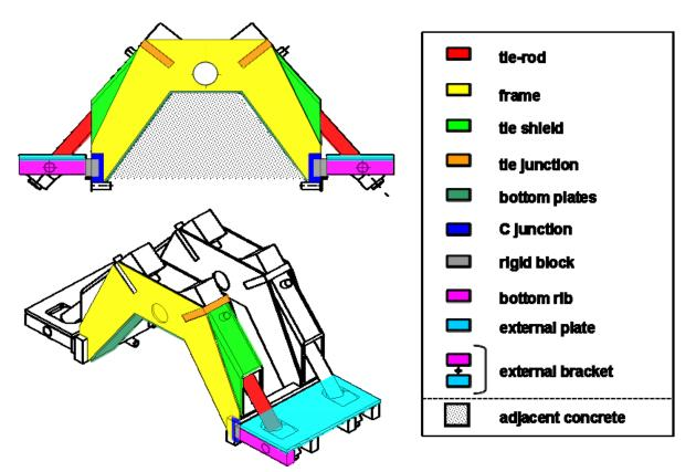
Fig.1: Structural decomposition of the cable-stayed innovative connection under study.
