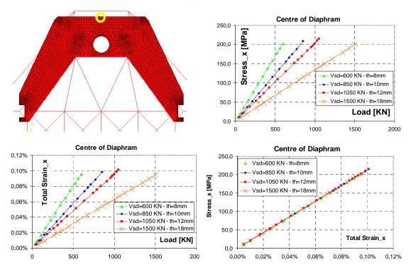
Fig.10: Load-stress and load strain diagrams under symmetric loading case (marked point).
