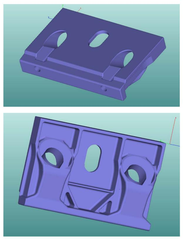
Fig.20: Top and bottom view of the finally obtained configuration of the external bracket.
