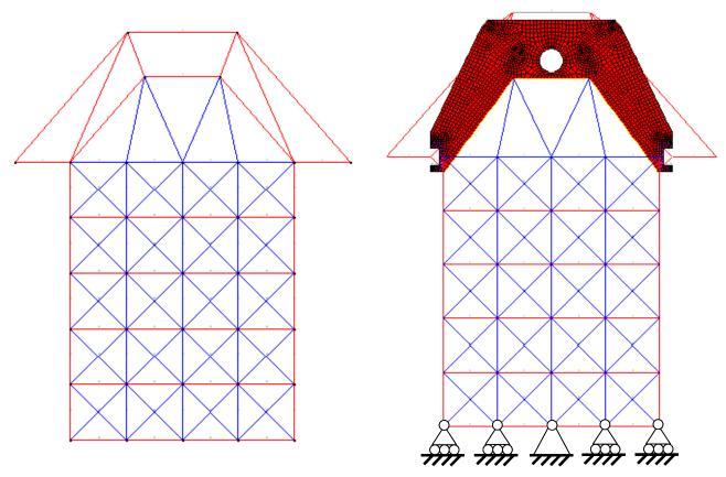
Fig.6: Full discrete (S&T) and mixed (FEM - S&T) modeling of the connection with base restraints.
