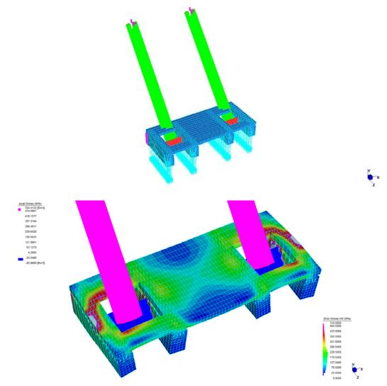
Fig.17: Initial configuration of the external part of the cable-stayed connection and, on the bottom, typical stress state after load application.
