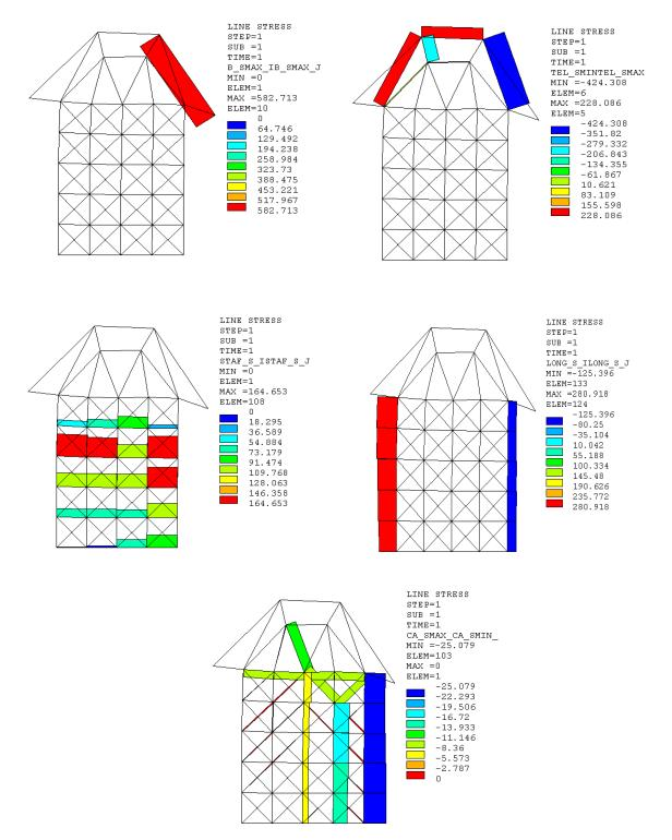
Fig.8: Typical results from S&T model: for the asymmetric load, on the top, axial actions on the bars representing the frame f the connection, in the middle stress on the stirrups and on the longitudinal bars, on the bottom, stress on the concrete core (please note the no tension response).
