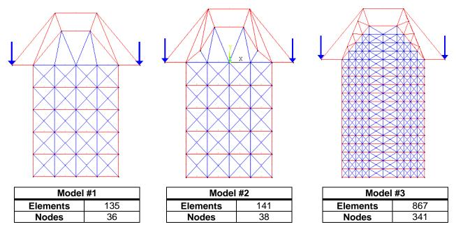
Fig.7: Aspect and characteristics of subsequent different S&T models.
