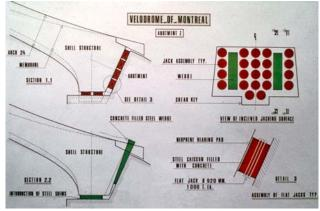
flat jack schematic at abutment Z
