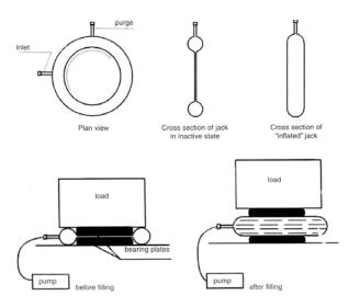
Figure 6 - Flat jack schematic
