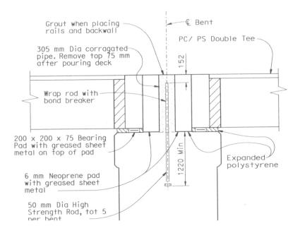
Fig. 8 Detail to Account for Sliding Movement at Bents 2 and 10.
