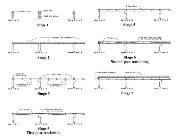
Fig. 7 Sequence of Construction Stages
