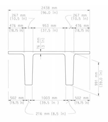
Fig. 6 Proposed Dimensions of Non-Standard Double Tee Girder.
