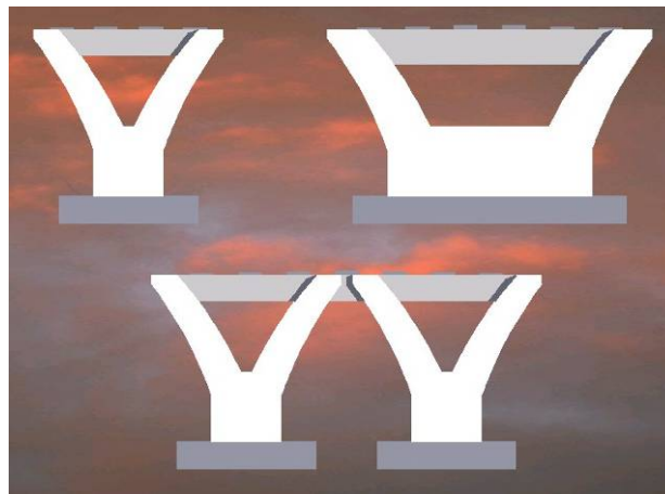
Fig. 5 Delta pier design variations
