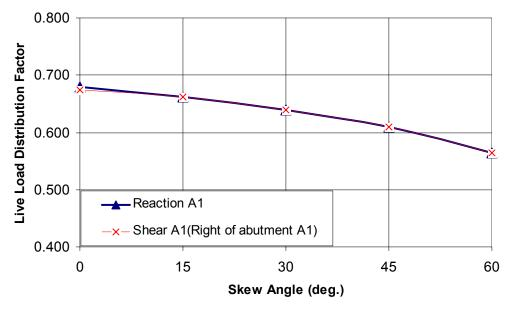
Fig. 6. Distribution Factors of Reaction and Shear at Support A1
