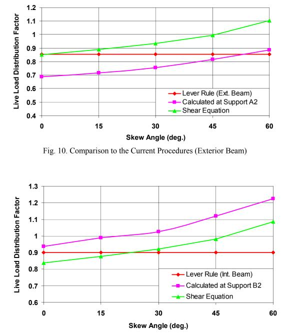
Fig. 11. Comparison to the Current Procedures (Interior Beam)
