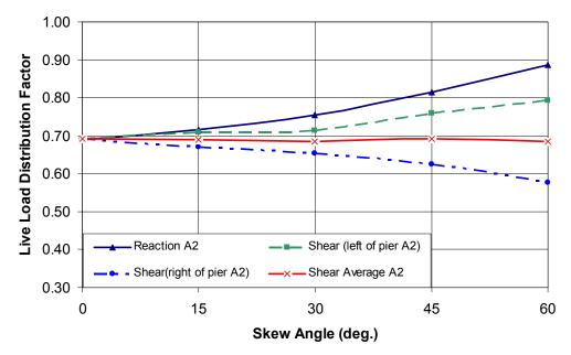
Fig. 7. Distribution Factors of Reaction and Shear at Pier A2
