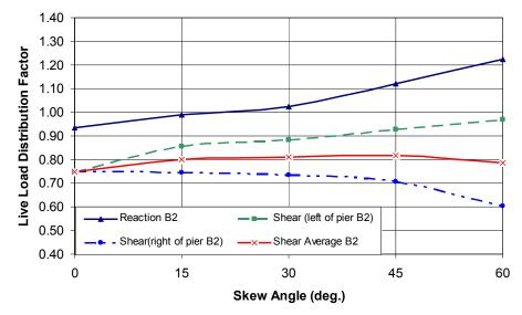
Fig. 8 Distribution Factors of Reaction and Shear at Pier B2
