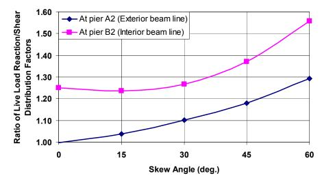
Fig. 9. Ratio of Reaction Distribution Factor vs. Shear Distribution Factor
