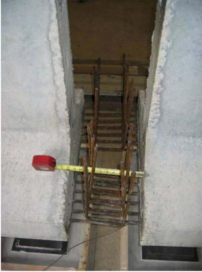
Fig. 6 Extended Strands for Test 1
