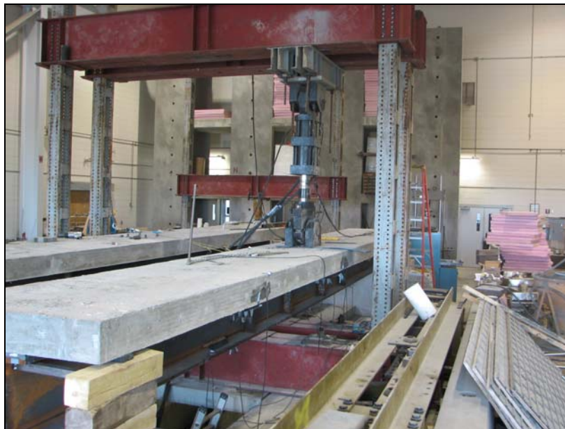
Figure 13. Fatigue test setup
