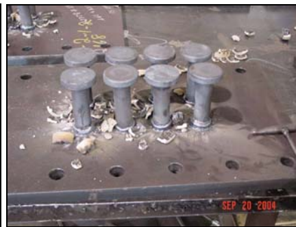
Figure 7. Fabrication of the push-off specimens
