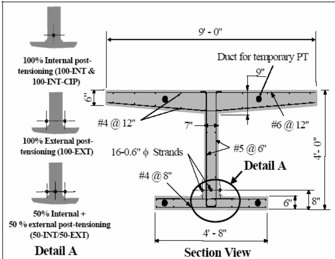
Fig. 3 Test Unit Cross Section
