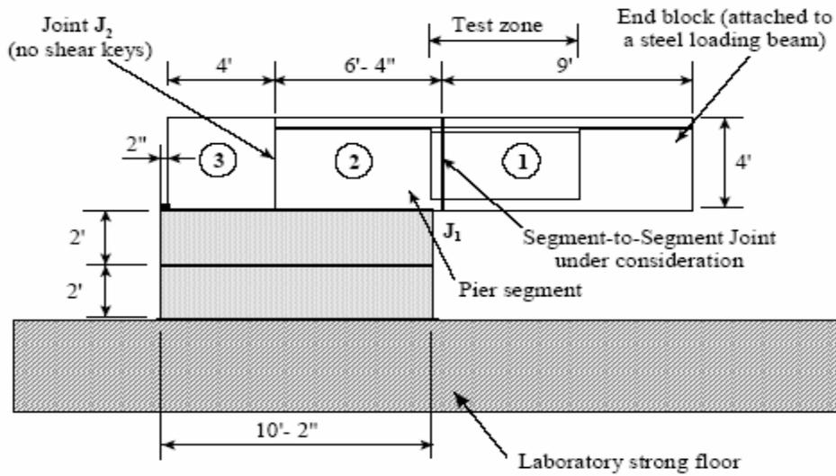
Fig. 6 Typical Test Unit Elevation
