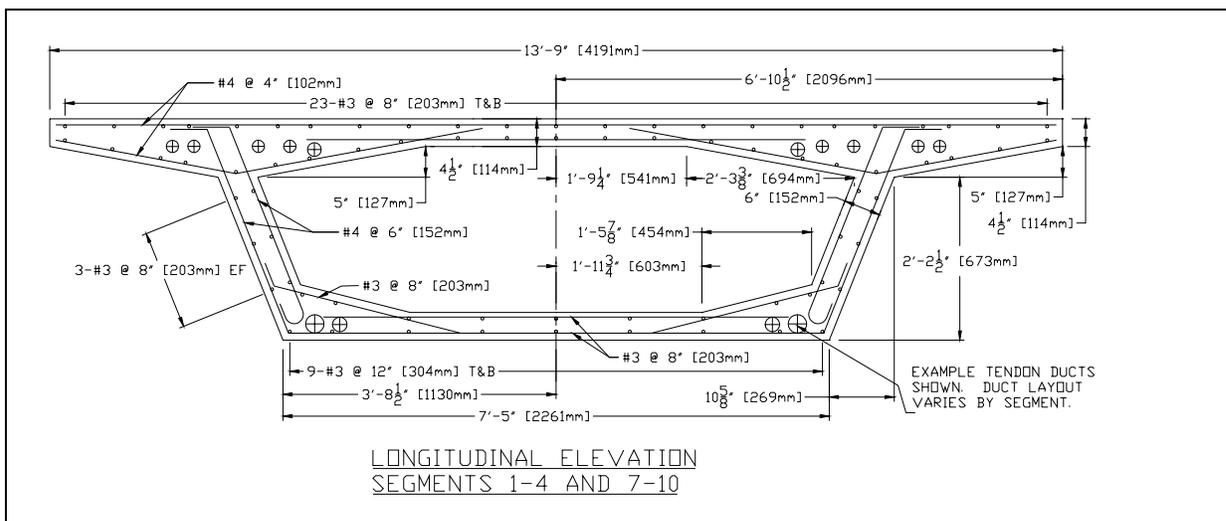
Fig. 9 System Test Cross Section
