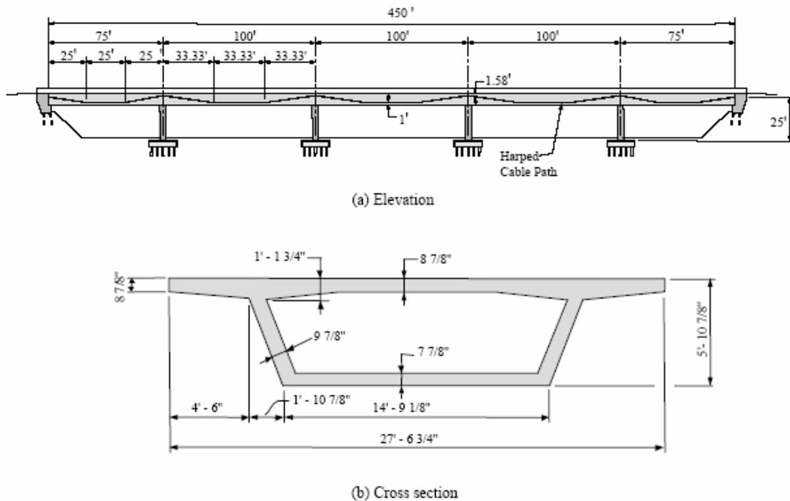
Fig. 1 Prototype Structure for Phase I and Phase II
