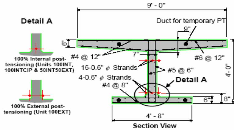
a) Cross Section of the Test Zone and the Horizontal Tendon
