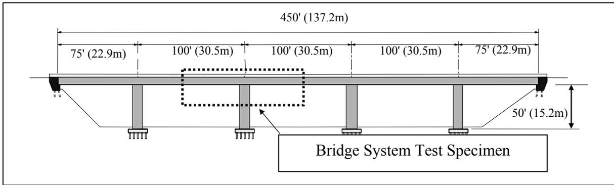
Fig. 7 Prototype Bridge Structure
