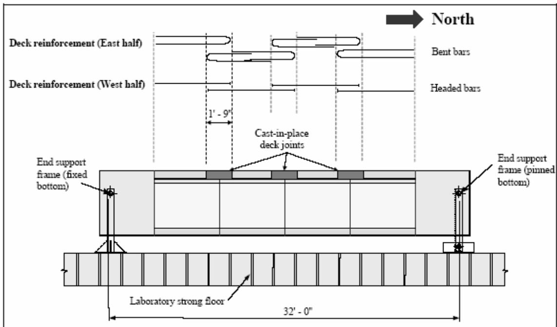
Fig. 4 Cast-in-place Deck Joint for Test Unit 100INTCIP
