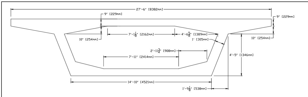
Fig. 8 Prototype box girder cross section
