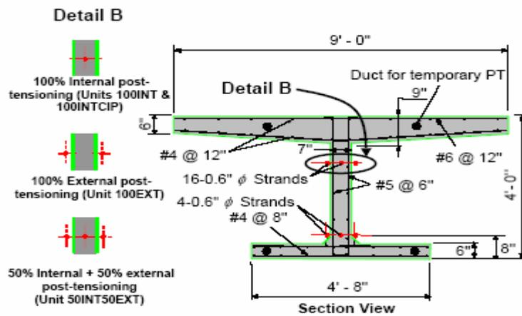
b) Cross Section of the Test Zone and the Harped-Shape Tendon
