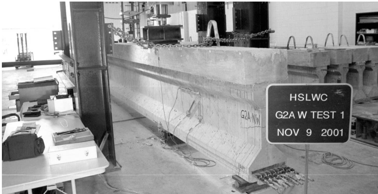
Fig. 1. West End of Girder G2A Before Development Length Testing
