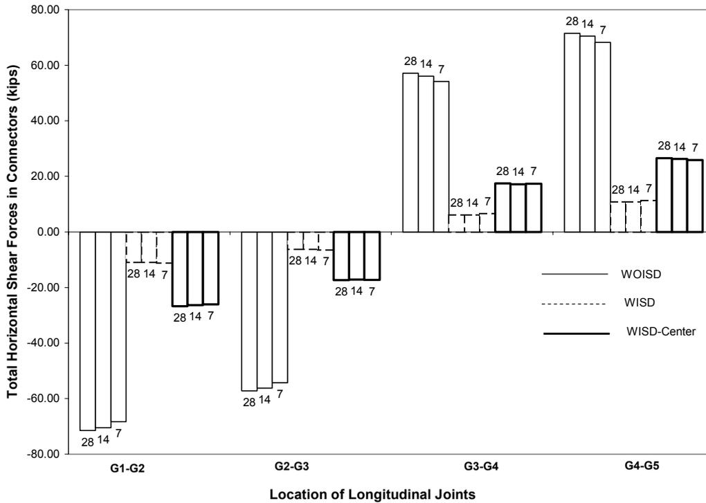
Fig. 21 Comparison of Total Horizontal Shear Forces in Connectors (“100<sup>th</sup> NB – 3 – G3”)
