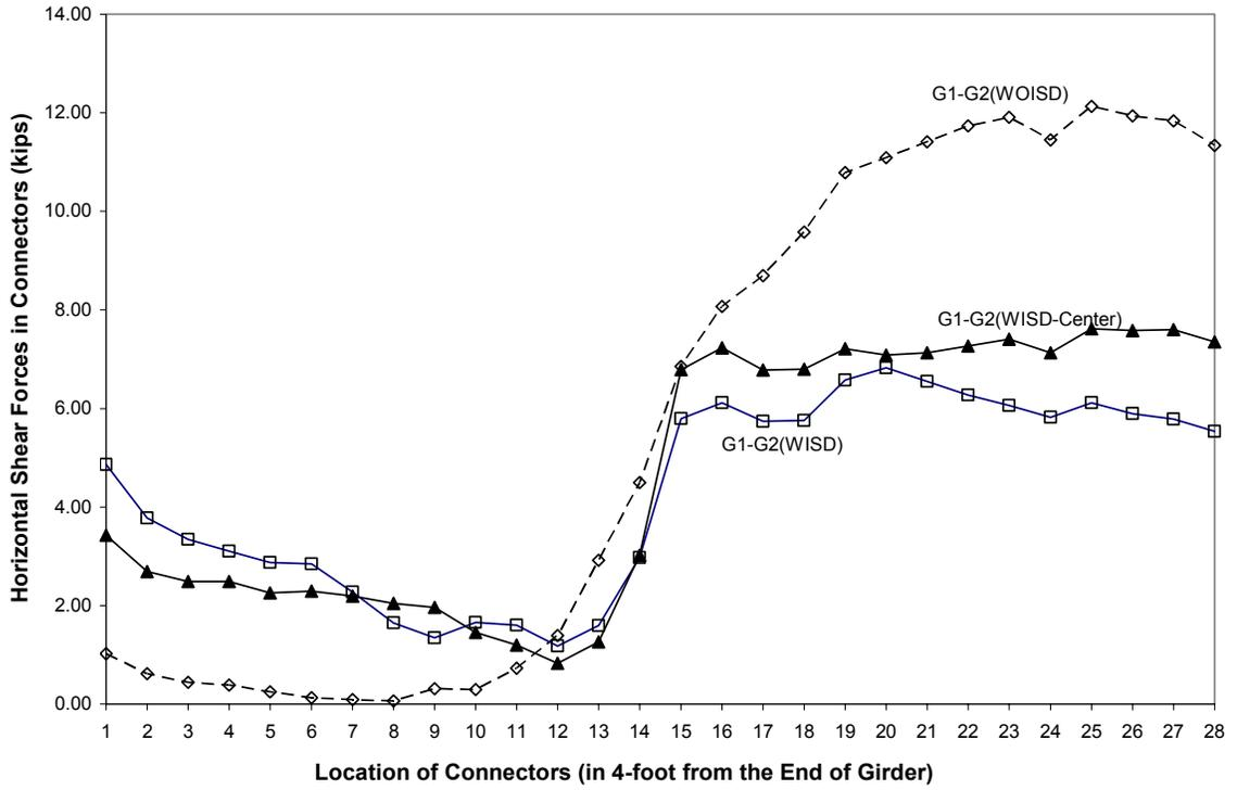
Fig. 13 Impact of Intermediate Diaphragm (“100<sup>th</sup> NB – 3 – G1”)
