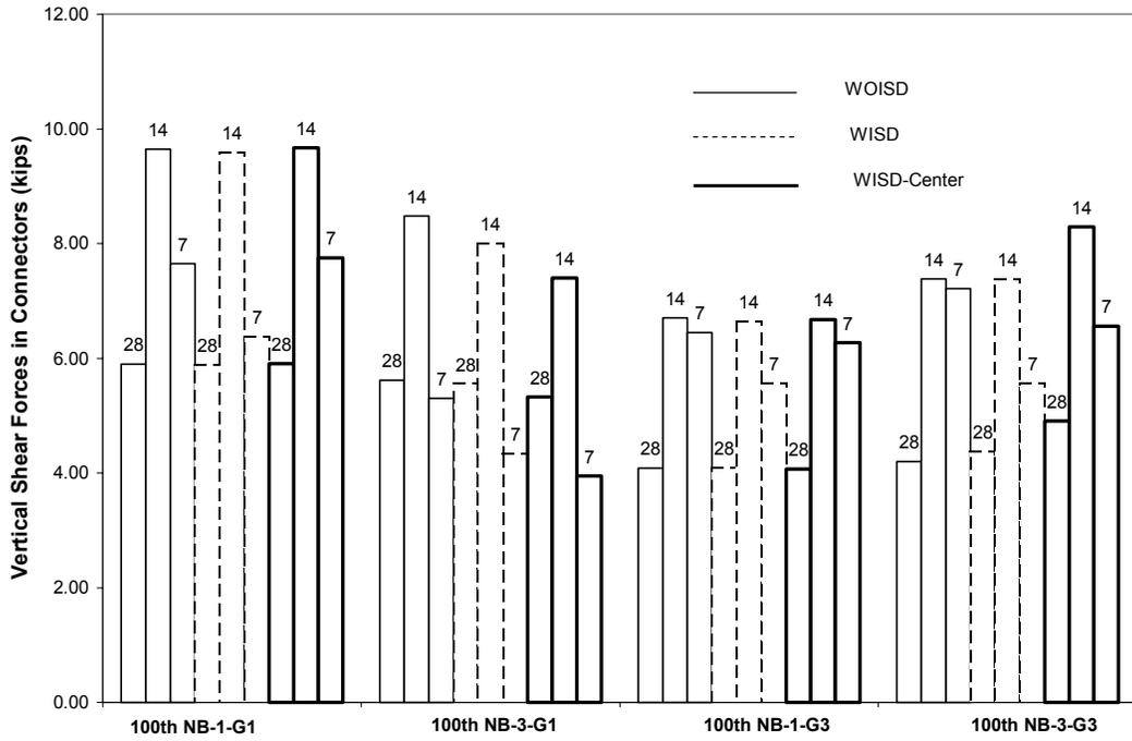
Fig. 19 Comparison of Maximum Vertical Shear Forces in Connectors
