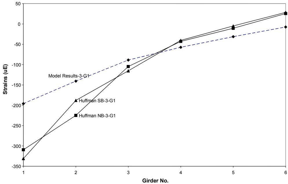
Fig. 7 Comparison of Flexural Strains for Huffman Bridge
