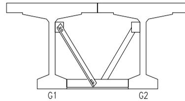
Fig. 2 Steel Diaphragms
