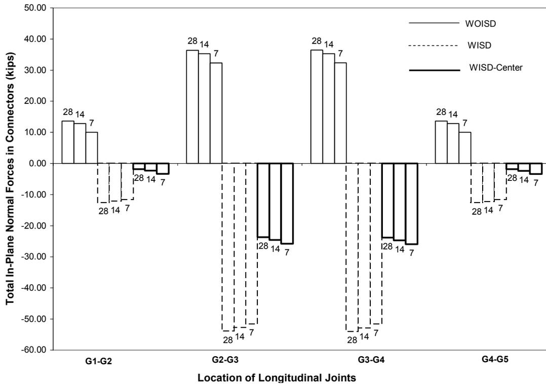
Fig. 23 Comparison of Total Normal Forces in Connectors (“100<sup>th</sup> NB – 3 – G3”)
