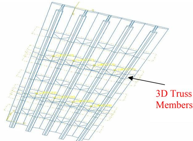
Fig. 3 Modeling Intermediate Steel Diaphragms
