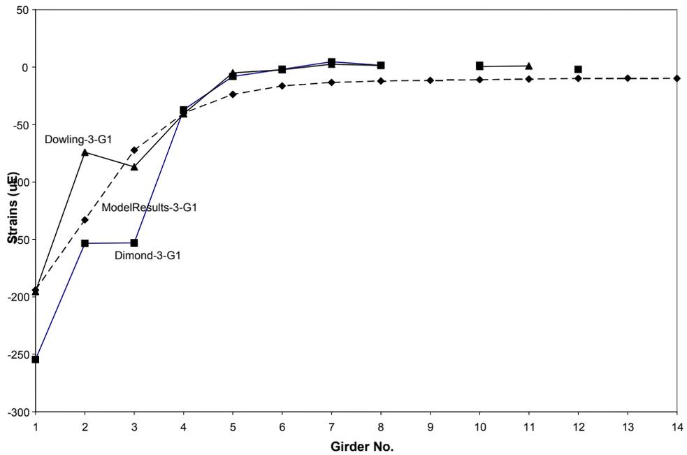
Fig. 5 Comparison of Flexural Strains for Dimond and Dowling Bridges
