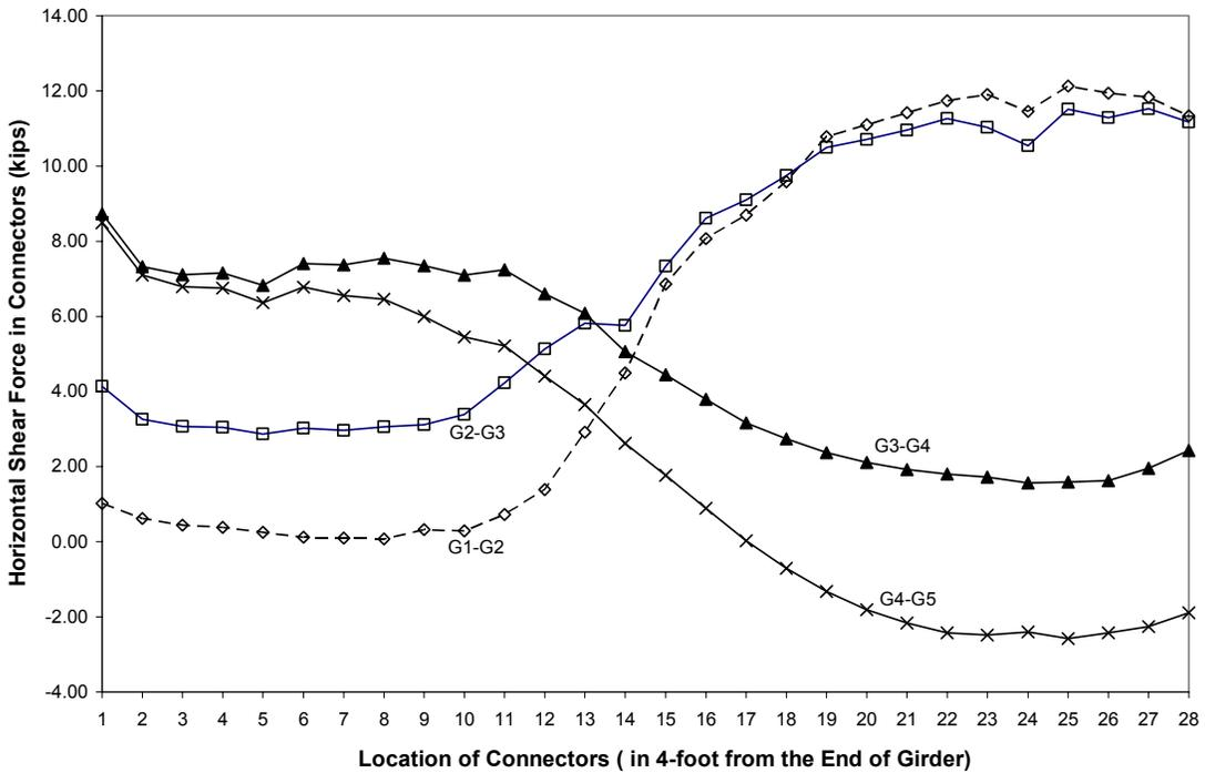
Fig. 14 Distribution of Horizontal Shear Forces in Connectors (“100<sup>th</sup> NB – 3 – G1”)
