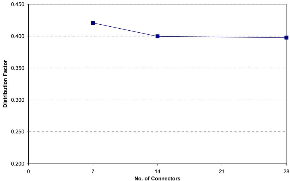
Fig. 10 Impact of Number of Shear Connectors on Distribution Factor
