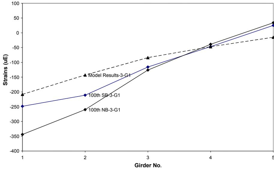
Fig.4 Comparison of Flexural Strains for 100<sup>th</sup> Bridge
