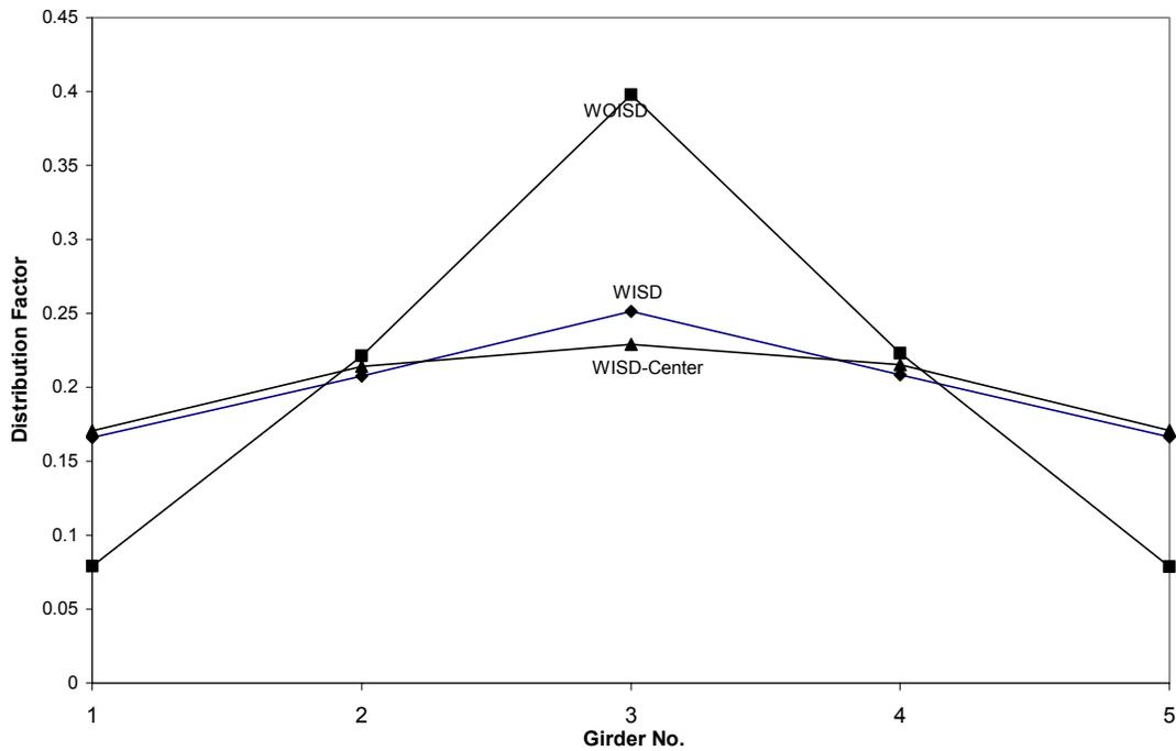
Fig. 9 Comparison of DF for Moment with Load at "100<sup>th</sup> NB - 3 - G3"
