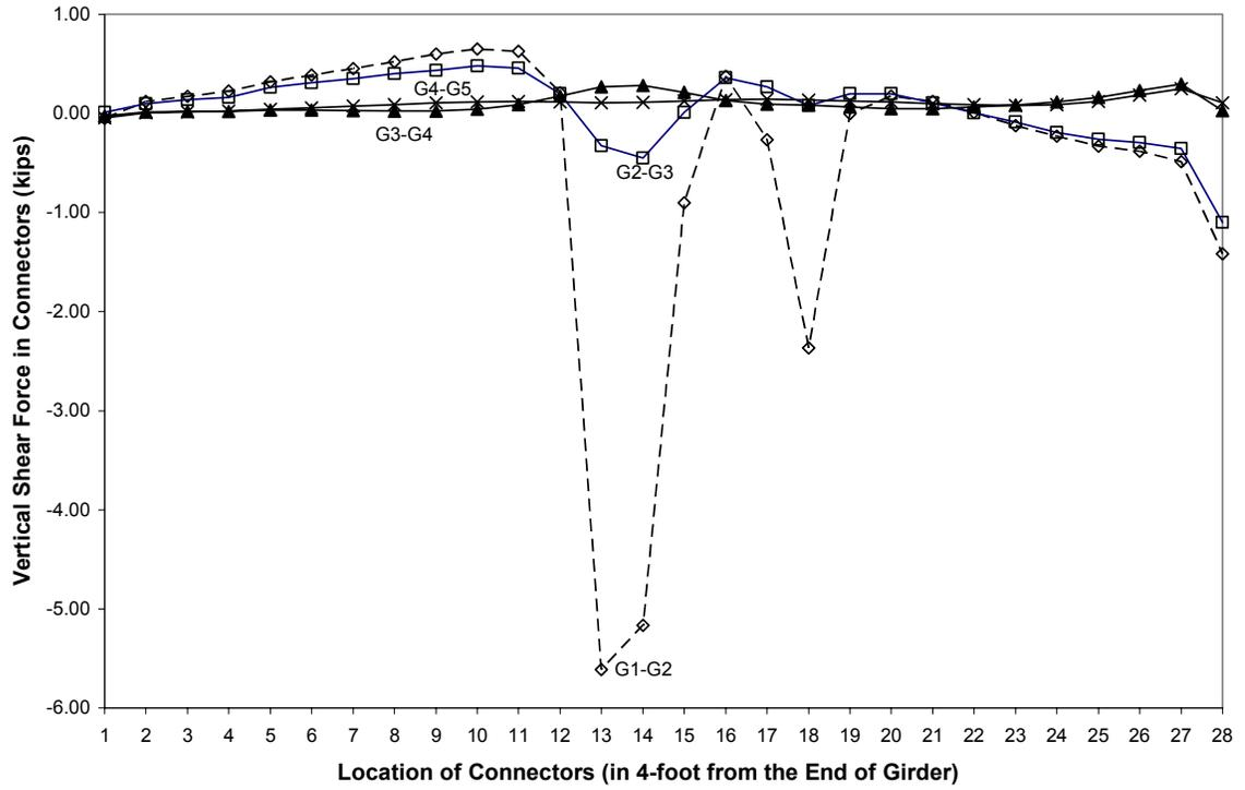
Fig. 15 Distribution of Vertical Shear Forces in Connectors (“100<sup>th</sup> NB – 3 – G1”)
