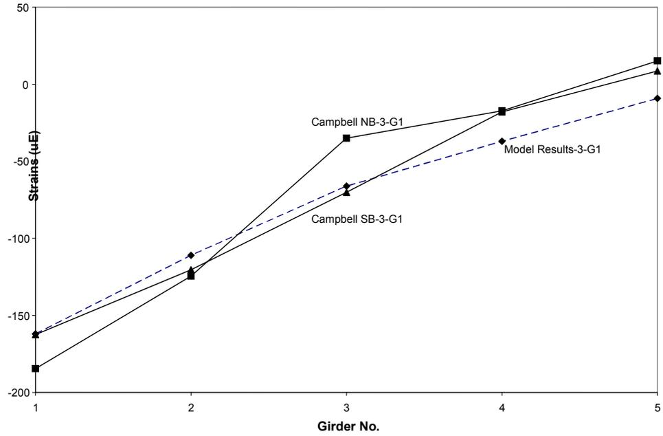
Fig.6 Comparison of Flexural Strains for Campbell Bridge
