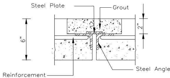
Fig. 1 Cross Section of the Shear Connector
