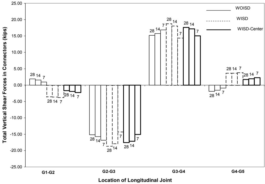
Fig. 22 Comparison of Total Vertical Shear Forces in Connectors (“100<sup>th</sup> NB – 3 – G3”)
