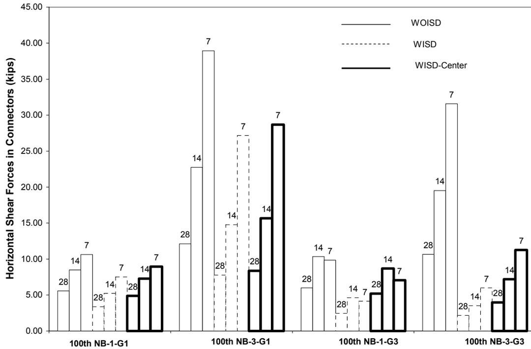
Fig. 18 Comparison of Maximum Horizontal Shear Forces in Connectors
