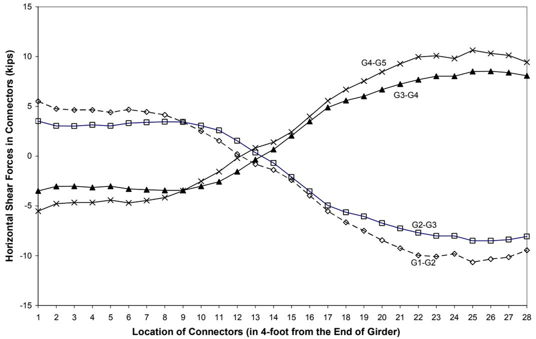
Fig. 16 Distribution of Horizontal Shear Forces in Connectors (“100<sup>th</sup> NB – 3 – G3”)
