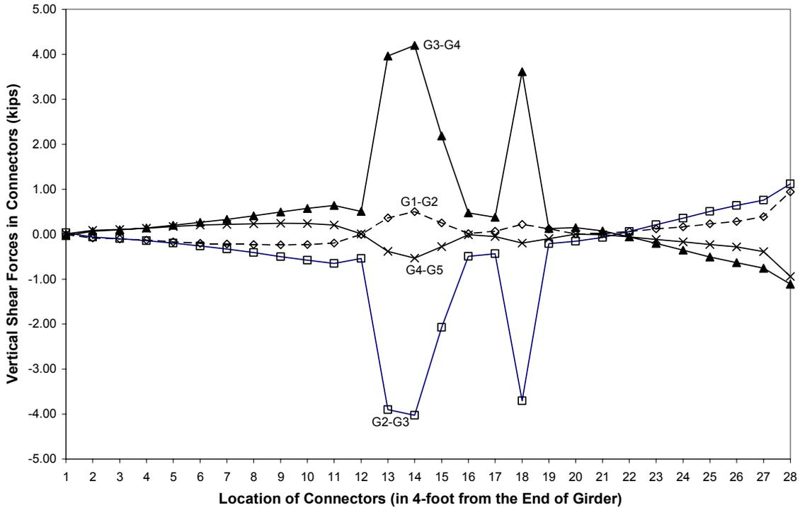
Fig. 17 Distribution of Vertical Shear Forces in Connectors (“100<sup>th</sup> NB – 3 – G3”)
