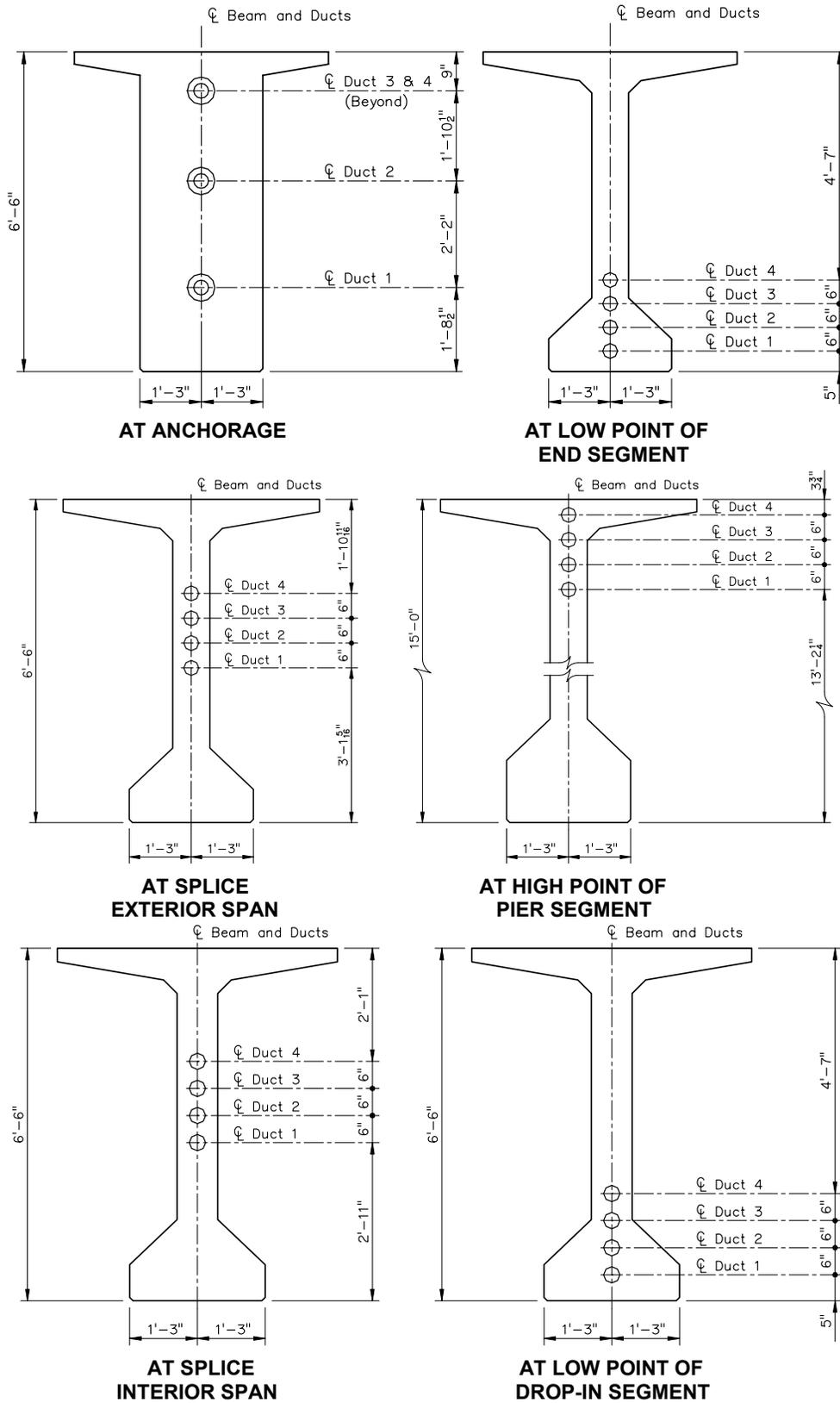
Figure 6 Duct Locations at Selected Sections Along the Bridge
