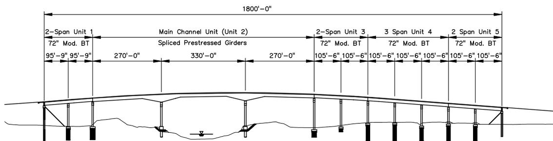
Figure 1 Elevation of Project
