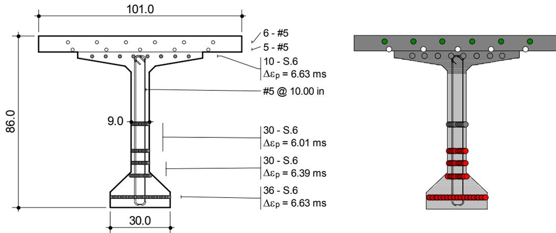
Figure 9 Example of Moment Curvature Analysis
