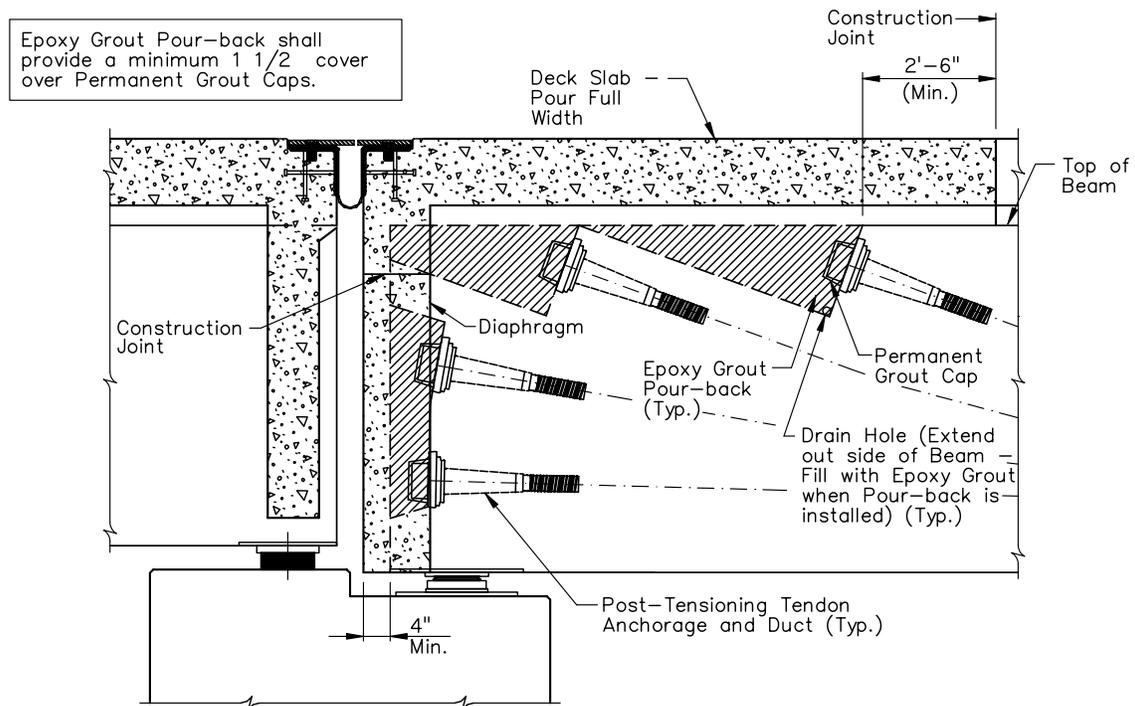
Figure 10 Details at Post-Tensioning Anchorages
