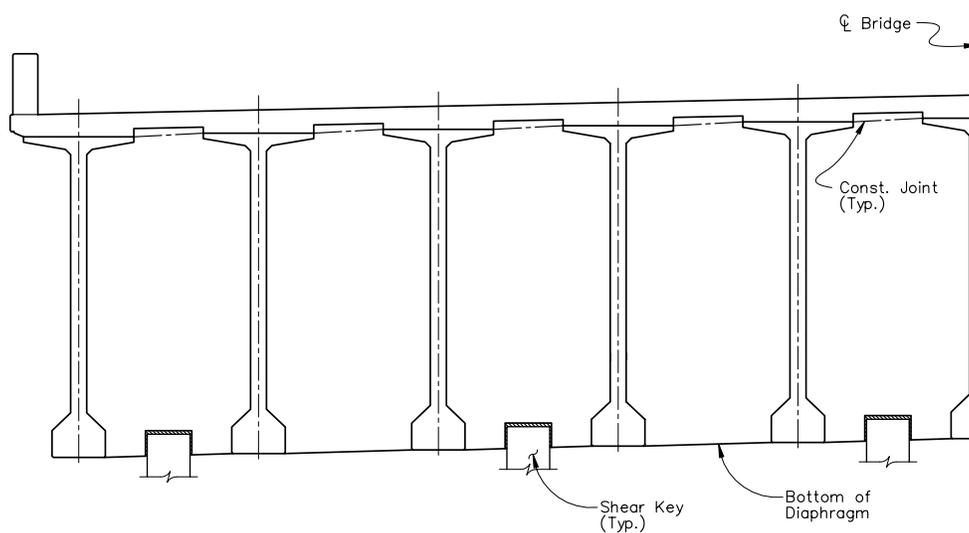
Figure 4 Typical Section at Interior Pier
