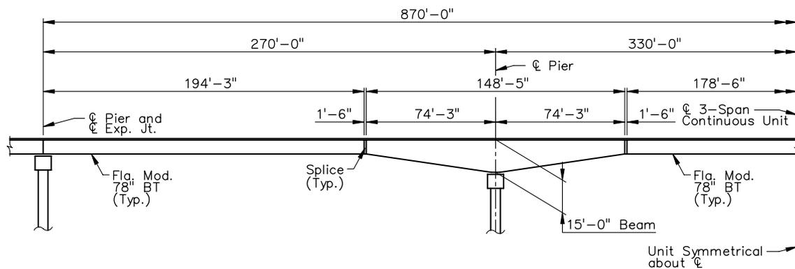
Figure 2 Half Elevation of Bridge Girder Layout
