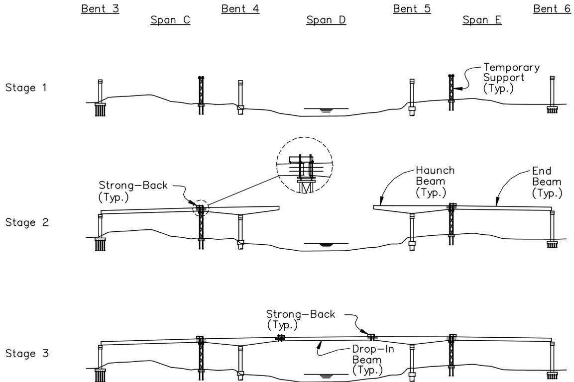
Figure 8 Girder Segment Erection Sequence
