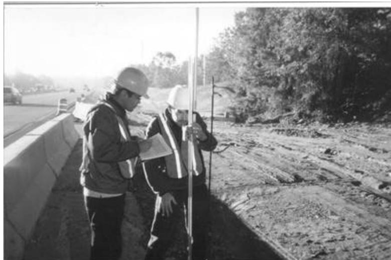
Figure 5. Photo of Deflection Rod Measurements.
