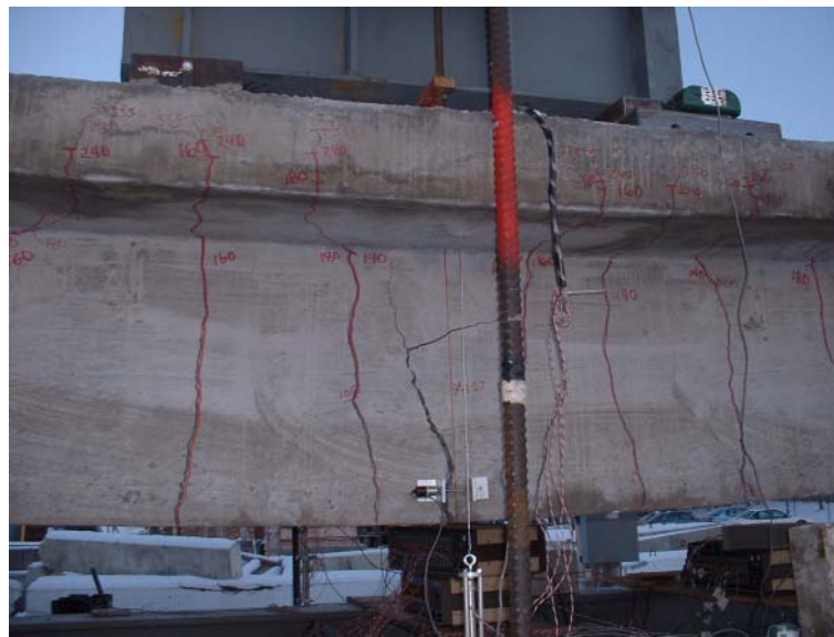
Figure 17. Ruptured FRP Deck Panel Stem
