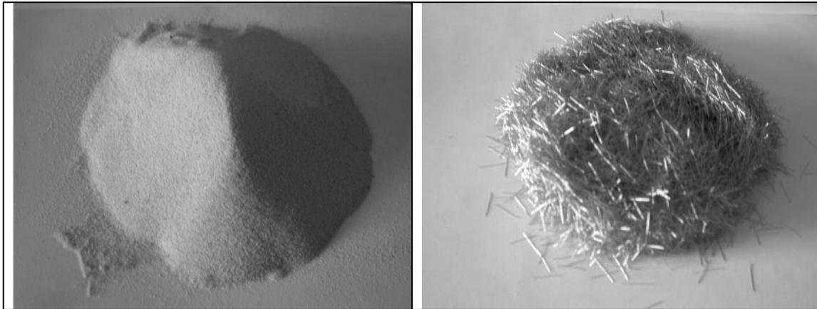
Fig. 6 and Fig. 7 Principal RPC components: quartz sand and steel fibers
