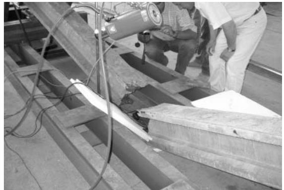
Fig. 14 and Fig. 15 Prestressed RPC beam load testing (Pojatno, May 2003)
