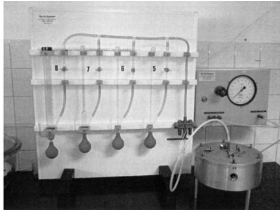
Fig. 19 Gas permeability testing equipment
