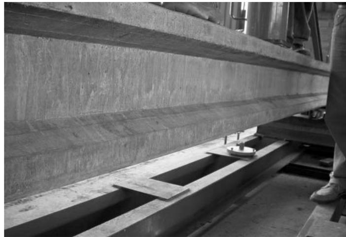
Fig. 12 and Fig. 13 Prestressed RPC beam (Pojatno, Croatia, May, 2003)
