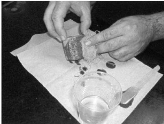
Fig. 18 Sample coating with epoxy resin
