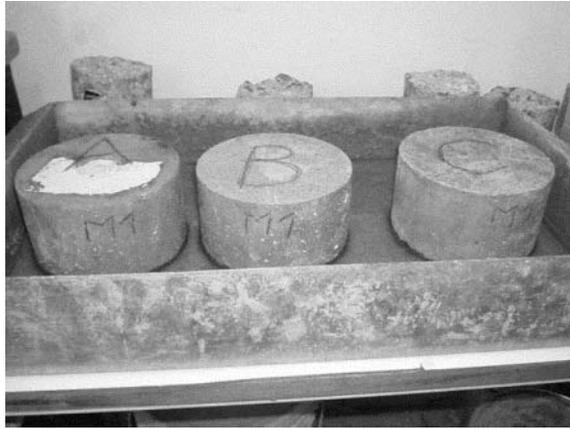
Fig. 20 Determination of water absorption by capillarity on concrete samples
