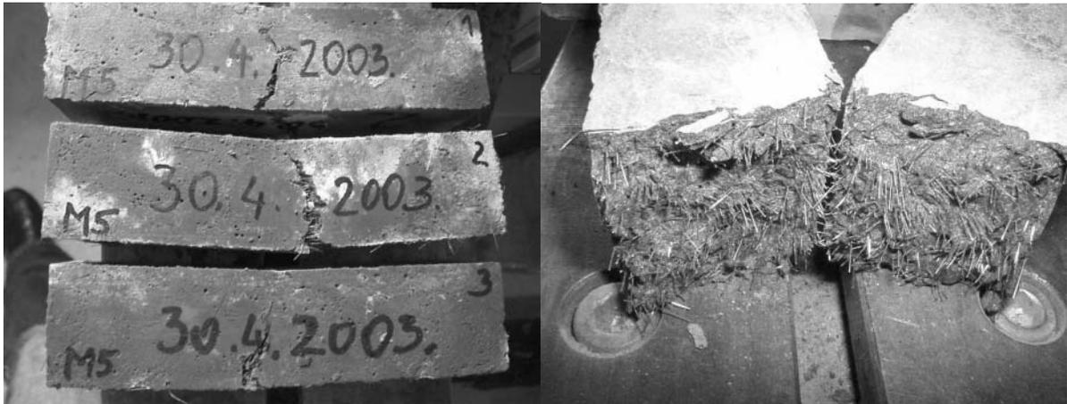
Fig. 16 and Fig. 17 View of prisms submitted to testing and prism cross section after failure
