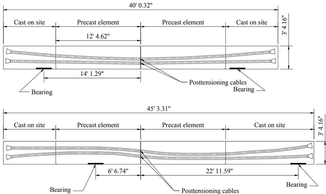
Fig. 4 Post-tensioning cables of the crossbeams at piers A (upper) and B (lower)
