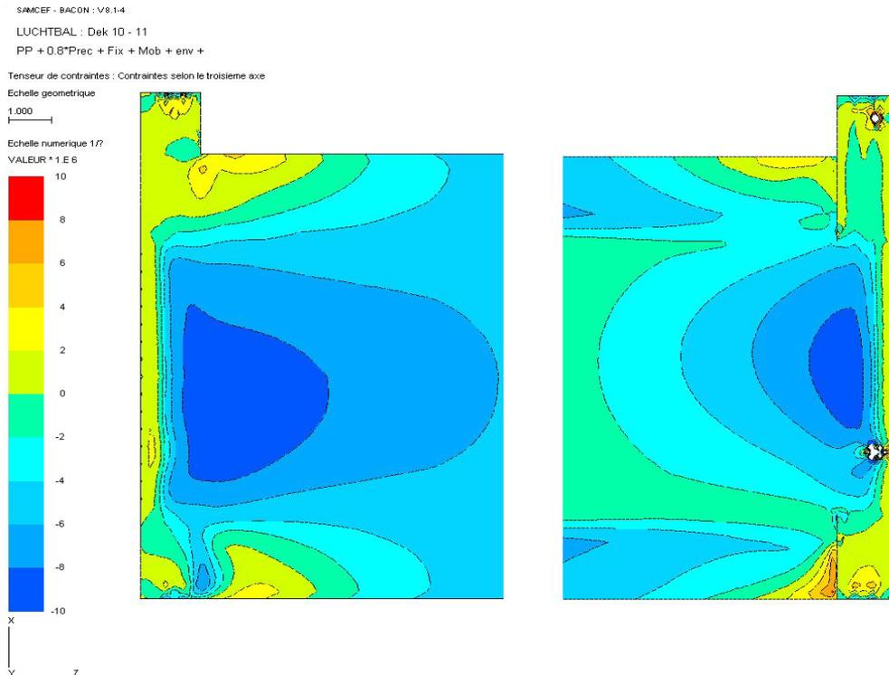
Fig. 11 Longitudinal stresses at the upper (left) and lower (right) surface (Color scale varies from -10 to +10 MPa or -1450 to 1450 psi)
