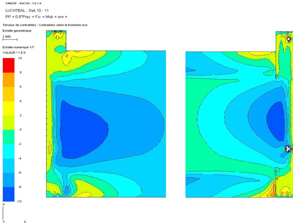
Fig. 11 Longitudinal stresses at the upper (left) and lower (right) surface (Color scale varies from -10 to +10 MPa or -1450 to 1450 psi)
