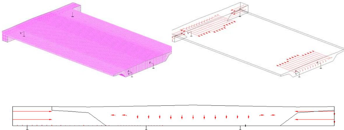
Fig. 9 Finite element model of the special decks near the crossing zone (upper left) with illustration of the vertical and horizontal forces at the end due to the post-tensioning (upper right) and more detailed in the cross section of the cantilever at the end (lower)
