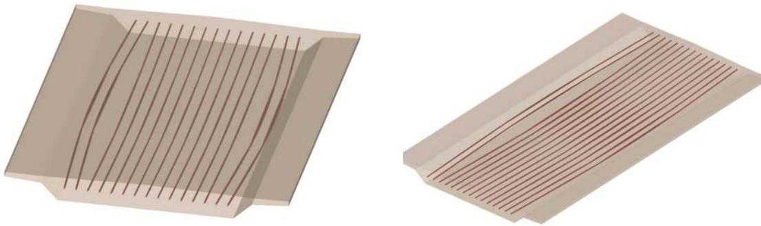
Fig. 8 View curved post-tensioning cables (left and right)
