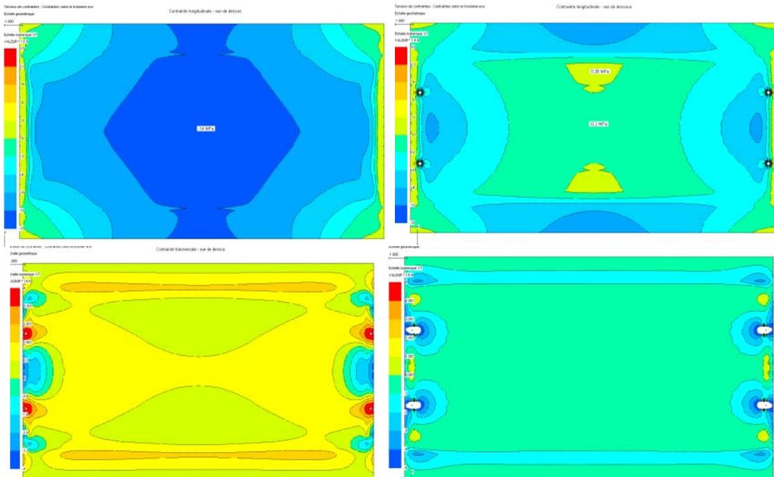
Fig. 7 Output of the finite element software: longitudinal normal stress at the upper fiber (upper left: -2176 psi to 2176 psi) and at the lower fiber (upper right: -2176 psi to 2176 psi) and transversal normal stress at the upper fiber (lower left: -580 psi to 580 psi) and at the lower fiber (lower right: -725 psi to 725 psi)
