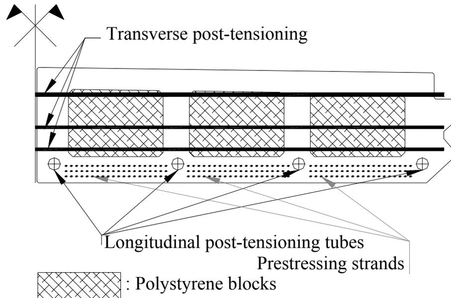
Fig. 3 Different types of tensioning in a typical precast element
