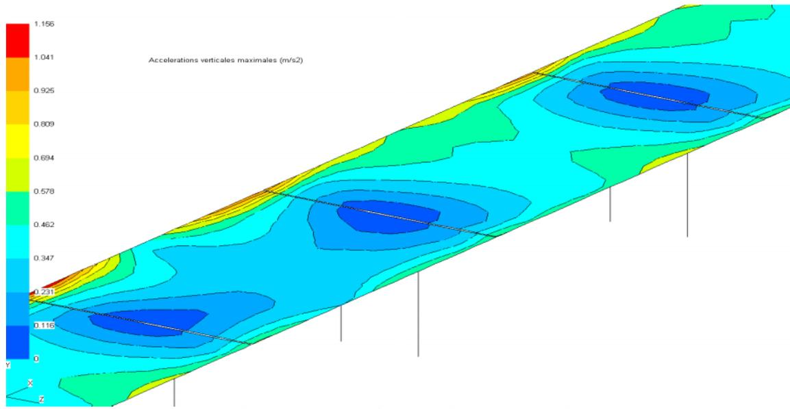
Fig. 13 Output of the vertical accelerations
