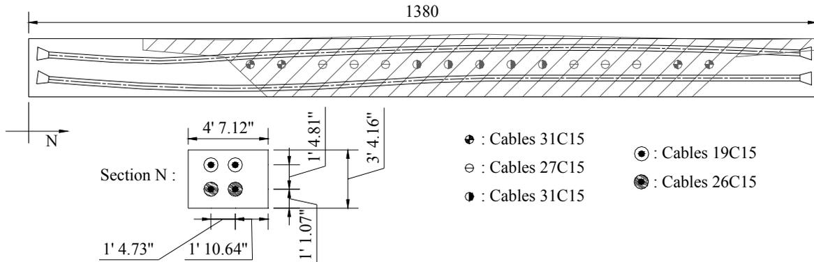
Fig. 10 Crossbeam for asymmetrical pier placement (pier type B)
