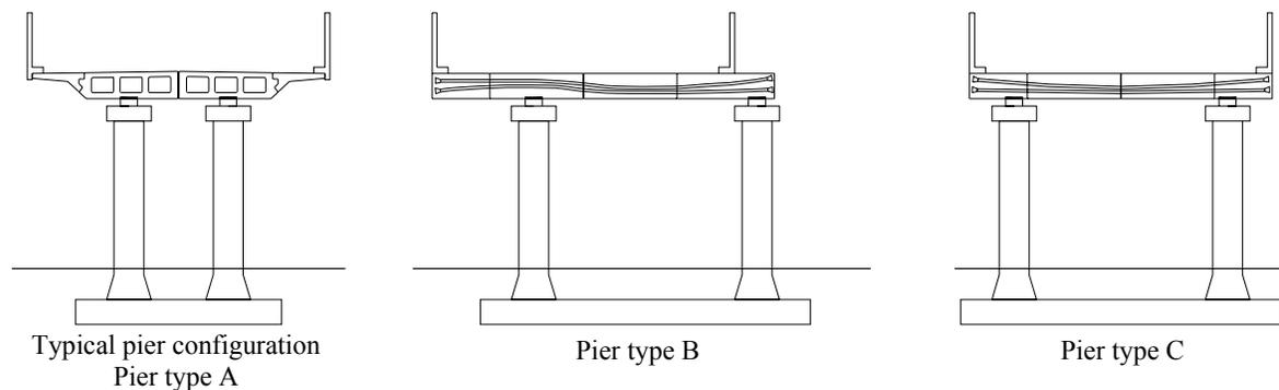
Fig. 5 Different pier configurations
