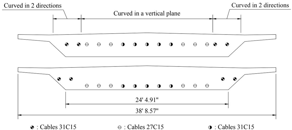
Fig. 6 Cross section at end span (upper) and mid span (lower)
