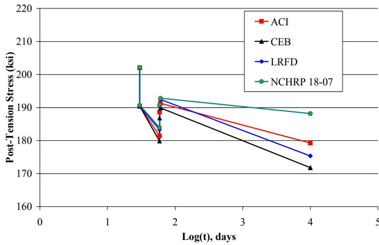
Fig. 10 Stress History in Post-Tensioning Tendons (Base Conditions; Cases 2, 5, and 8)
