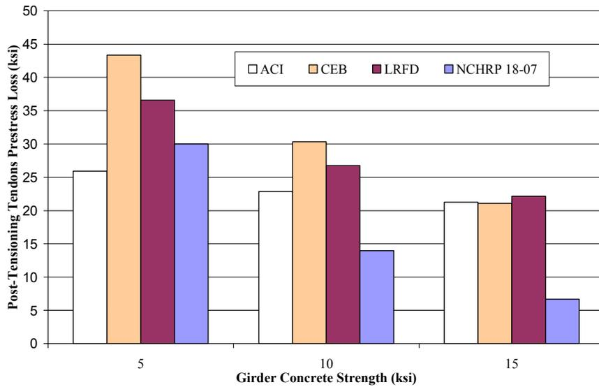
**Fig. 13 Post-Tensioning Tendons Prestress Loss for Varying Girder Concrete Strengths Using Various Methods**
