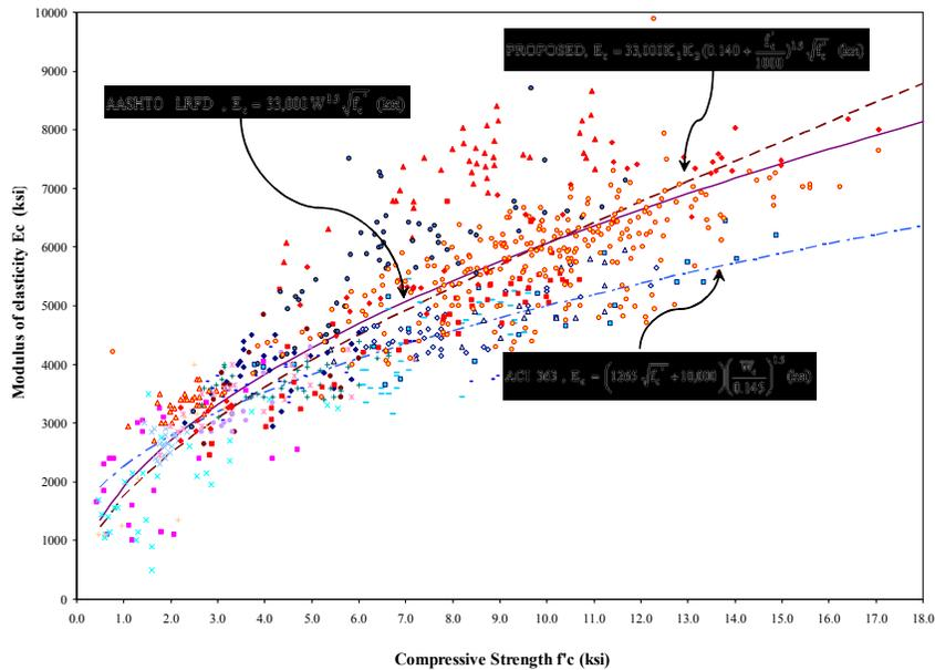
Fig. 1 NCHRP 18-07 Modulus of Elasticity Test Results
