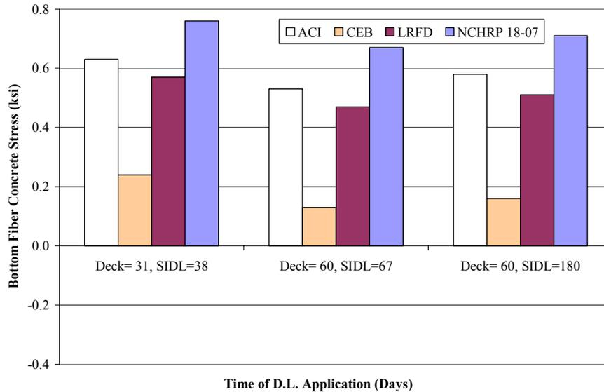
**Fig. 16 Bottom Fiber Concrete Stress Varying the Time of Applying the SIDL**
