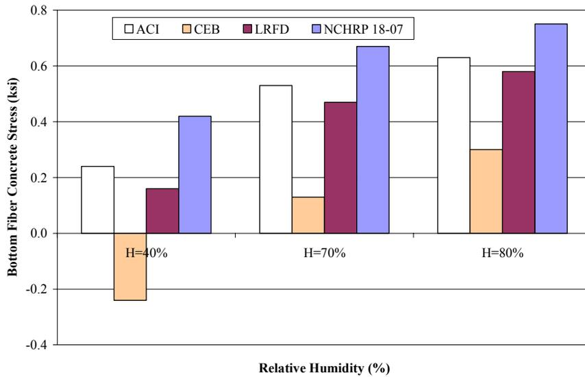
Fig. 15 Bottom Fiber Concrete Stress for Various Levels of Relative Humidity
