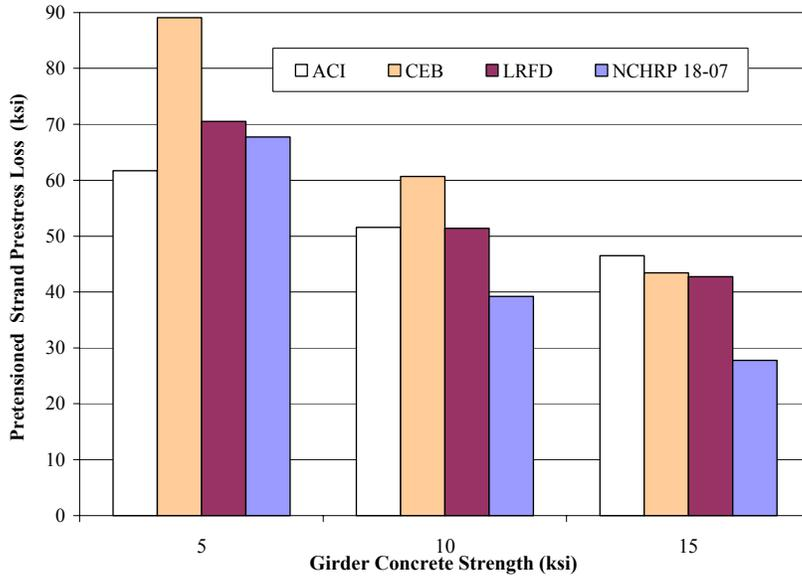
**Fig. 12 Pretensioned Strand Prestress Loss for Varying Girder Concrete Strengths Using Various Methods**
