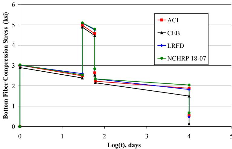
Fig. 11 Stress History in Bottom Fiber Concrete (Base Conditions; Cases 2, 5, and 8)
