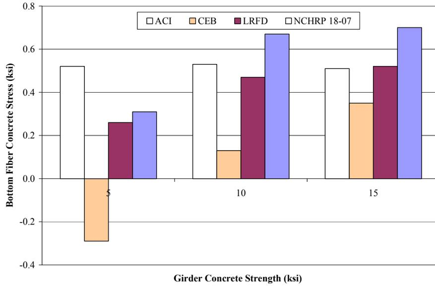
Fig. 14 Bottom Fiber Concrete Stress for Varying Girder Concrete Strengths Using Various Methods
