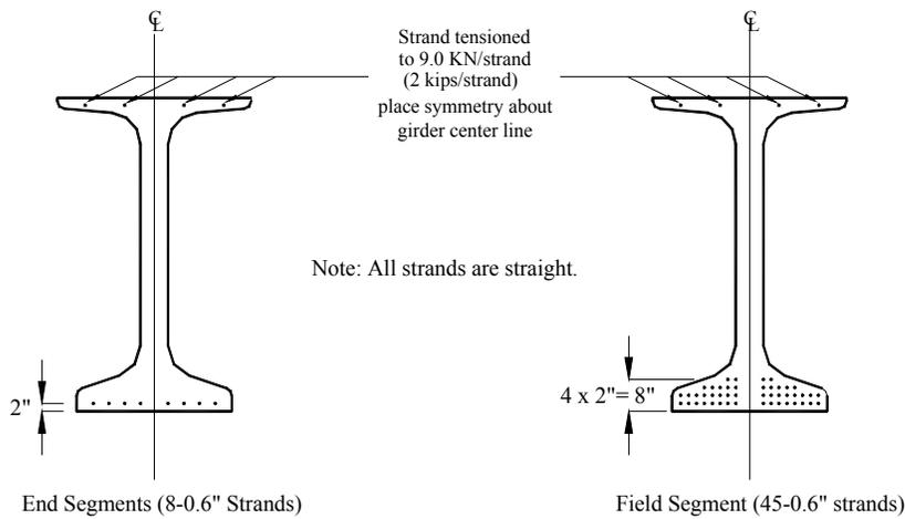
**Fig. 7 Pretensioning Scheme of the 198<sup>th</sup> – Skyline Drive Bridge**
