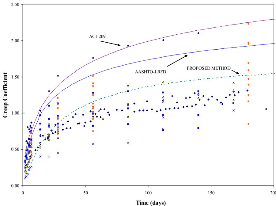
Fig. 3 NCHRP 18-07 Creep Coefficient Test Results (Specimens Loaded at 1 Day)
