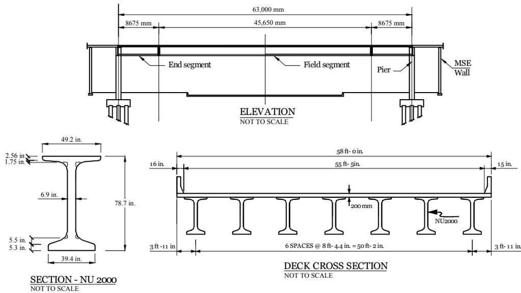
**Fig. 5 General Layout of the 198<sup>th</sup> – Skyline Drive Bridge**
