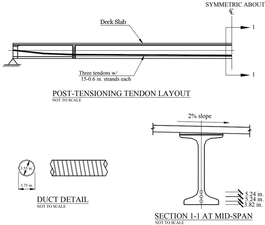
**Fig. 8 Post-tensioning Details of the 198<sup>th</sup> – Skyline Drive Bridge**
