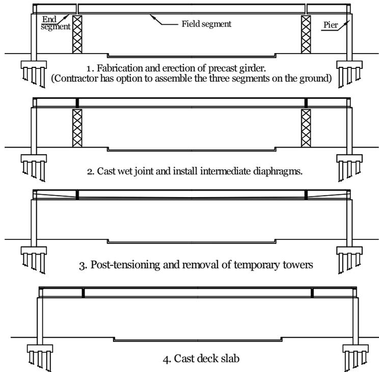
**Fig. 6 Construction Sequence of the 198<sup>th</sup> – Skyline Drive Bridge**
