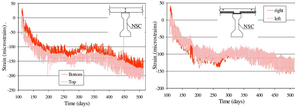
Fig. 11 Measured Time-Dependent Concrete Strains in Deck (0.4L Section) of NSC Bridge
