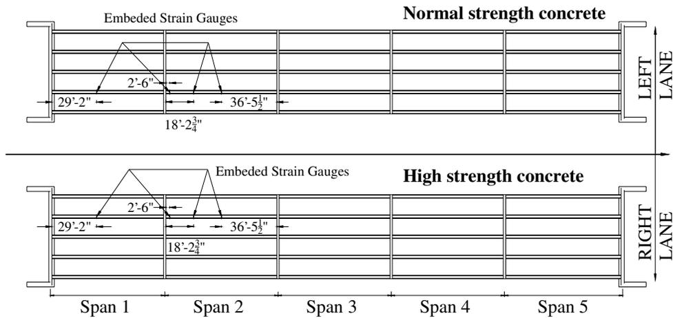
Fig.2 Plan View of Bridge Instrumentation
