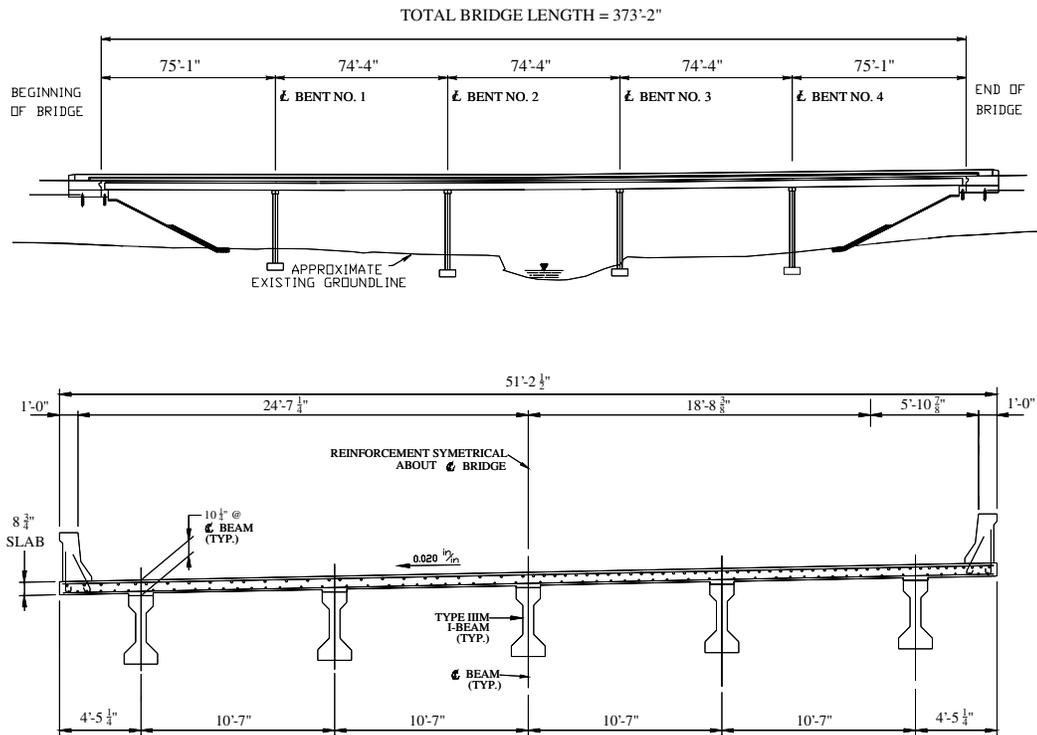
Fig. 1 Elevation and Typical Cross-section of Pistol Creek Bridge
