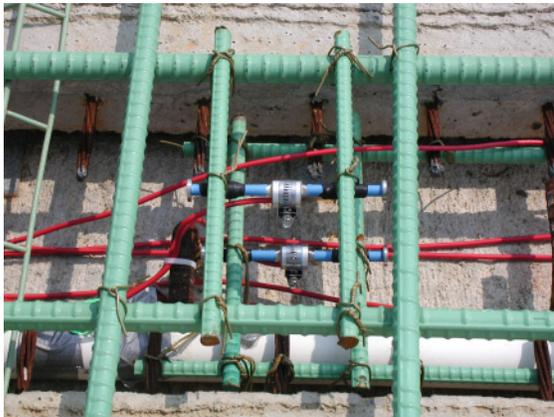
(a) Strain gauges over beam
