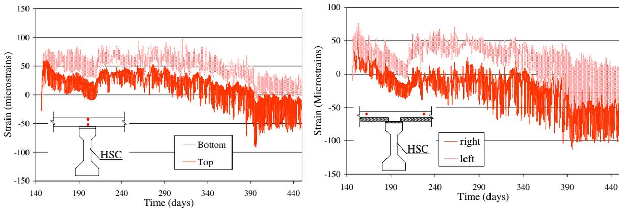
Fig. 12 Measured Time-Dependent Concrete Strains in Deck (0.4L Section) of HSC Bridge
