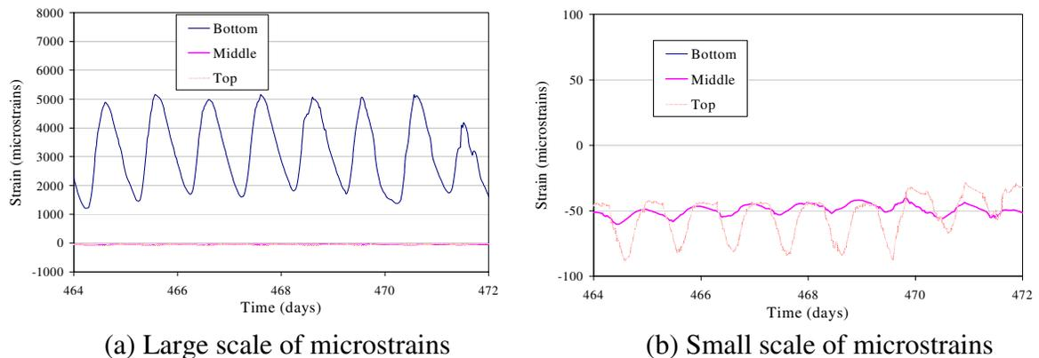
Fig. 13 Measured Strains Variation in the Diaphragm (NSC Bridge)
