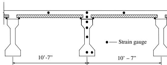
Fig. 3 Gauge Positions in Precast Beam and Deck Slab
