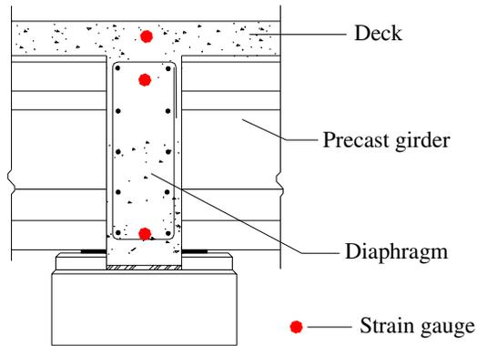
Fig. 4 Gauge Positions in Diaphragm
