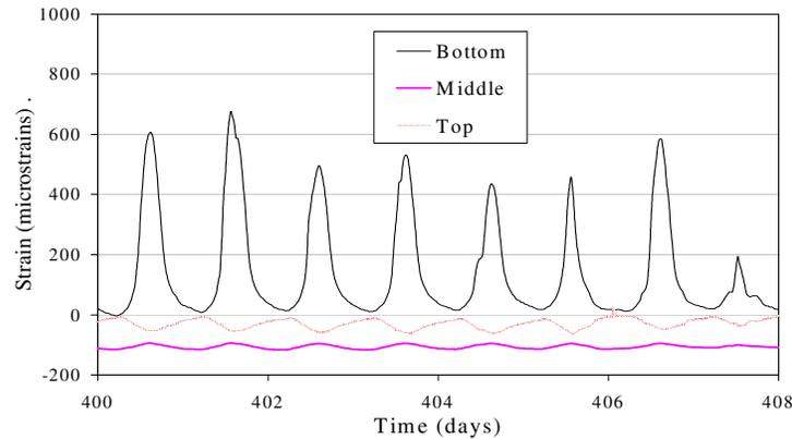
Fig. 14 Measured Strains Variation in the Diaphragm (HSC Bridge)
