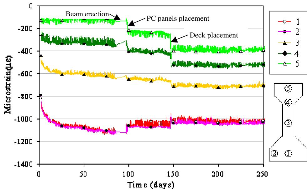
Fig. 9 Measured Time-Dependent Concrete Strains at Midspan Section of HSC
