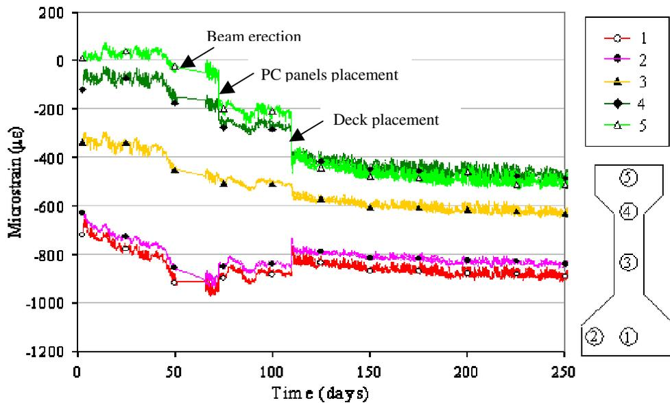
Fig. 8 Measured Time-Dependent Concrete Strains at Midspan Section of NSC
