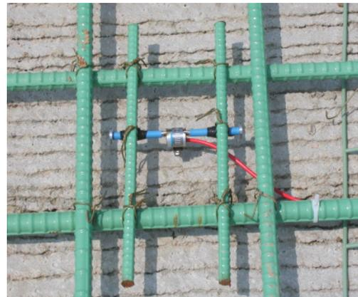
(b) Strain gauges over precast panel
