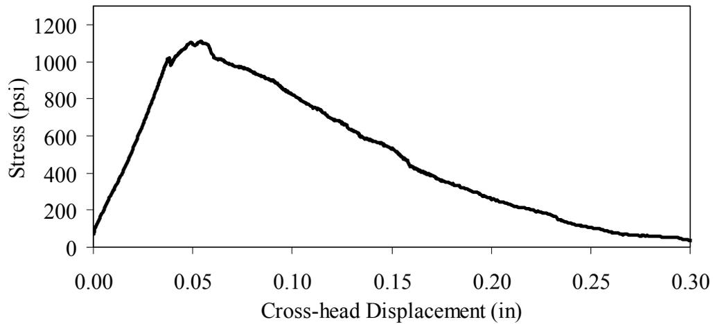
Figure 2. Load-Displacement Response for a Steam Cured Mortar Briquette.
