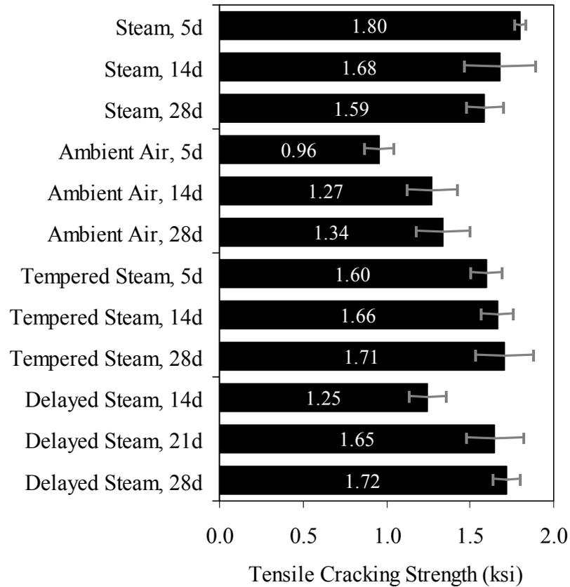
Figure 5. Split Cylinder Tensile Cracking Strength.
