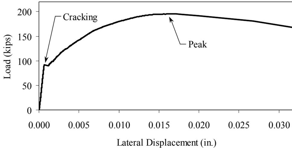
Figure 4. Split Cylinder Lateral Deflection Response for a Steam Cured Specimen.
