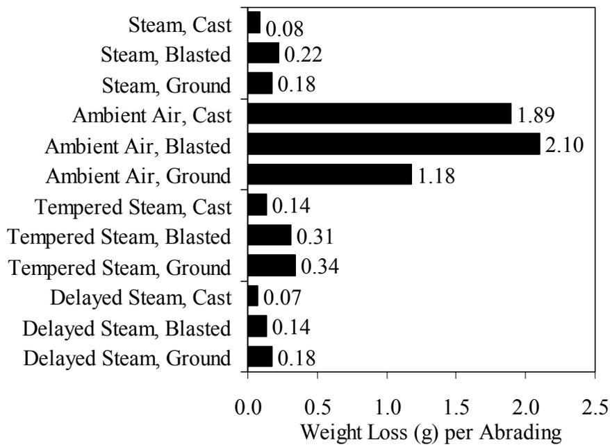
Figure 9. ASTM C944 Abrasion Resistance.
