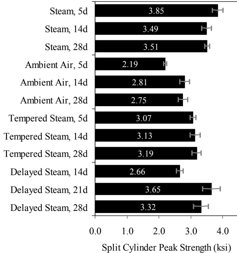
Figure 6. Split Cylinder Peak Strength.
