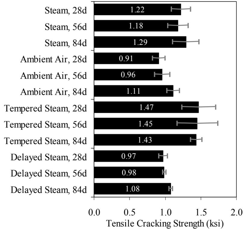
Figure 1. Mortar Briquette Tensile Cracking Strength.
