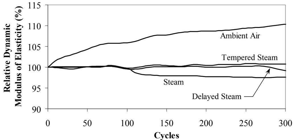
Figure 10. Freeze-Thaw Resistance of UHPC.
