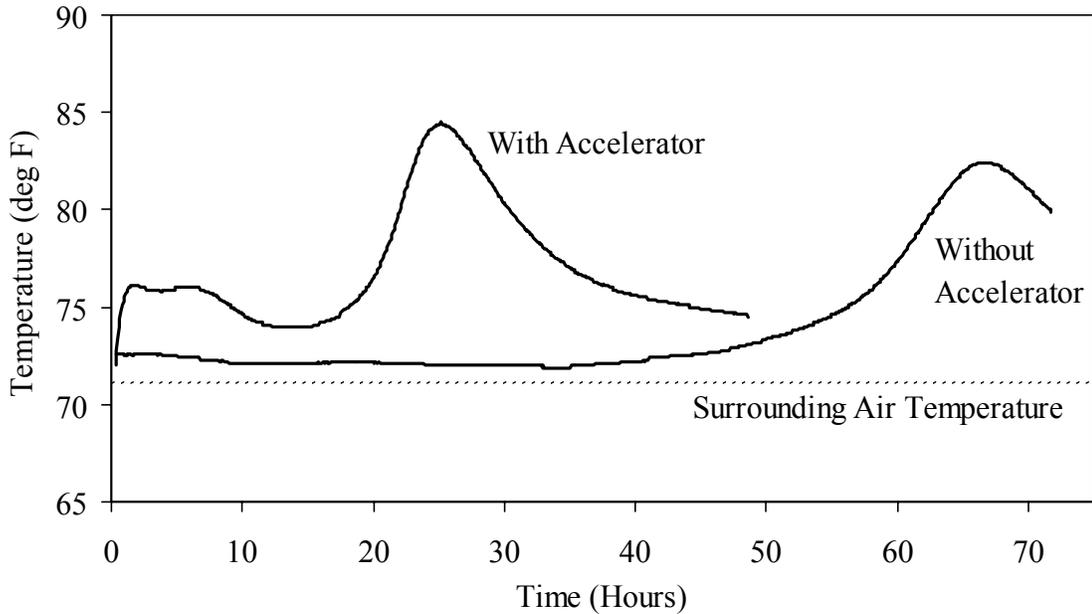
Figure 7. Temperature in a 6x12 in. Cylinder With and Without Accelerator in Mix.
