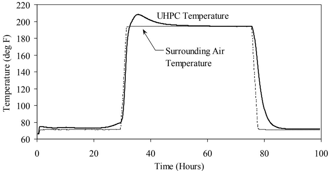
Figure 8. Temperature in a 6x12 in. Cylinder from Casting through Steam Curing.
