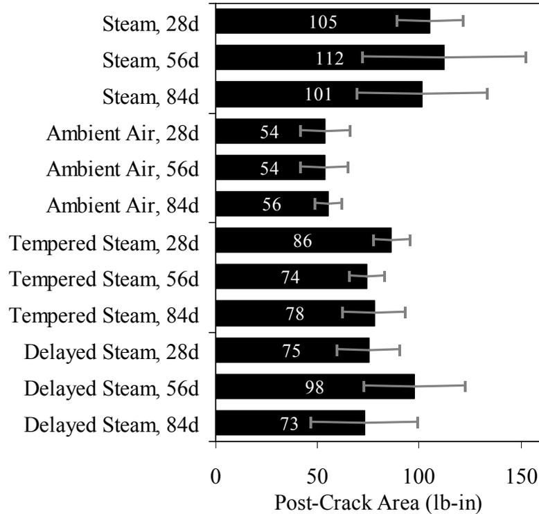
Figure 3. Area Under Mortar Briquette Load-Deflection Curve After Cracking.
