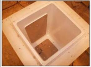
Fig. 13 Inside of mould, showing openings for the top and rear doors
