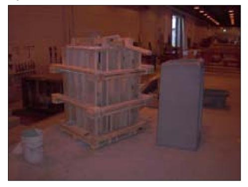
Fig. 15 Form and prototype waste container
