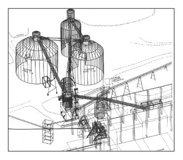
Fig. 2 Schematic : General arrangements – clinker storage & handling
