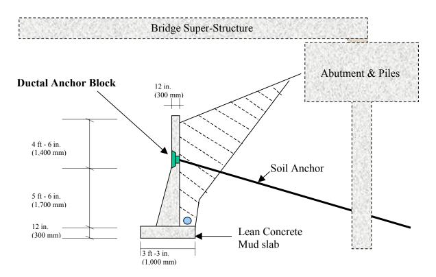
Fig. 17 Schematic of retaining wall with precast anchor blocks
