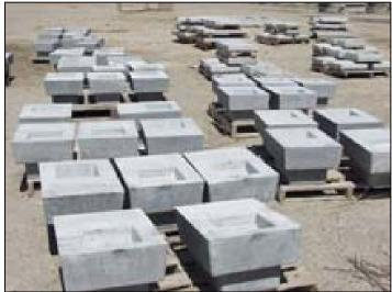
Fig. 20 Anchor blocks ready for shipping
