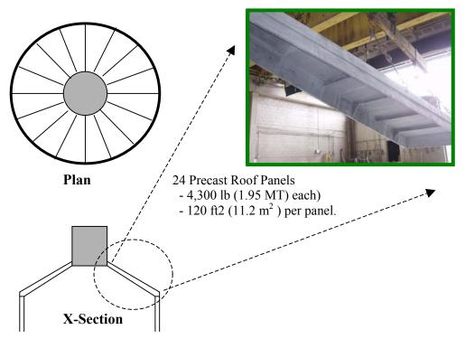
Fig. 3 Plan and section of the clinker storage silo
