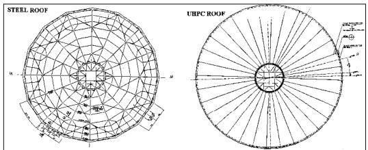
Fig. 5 Steel framing (left) vs. precast framing (right) for the silo roof
