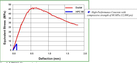
Fig. 1 UPHC Stress-strain curve
