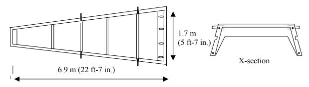
Fig. 4 Sketch of the panel for the silo roof
