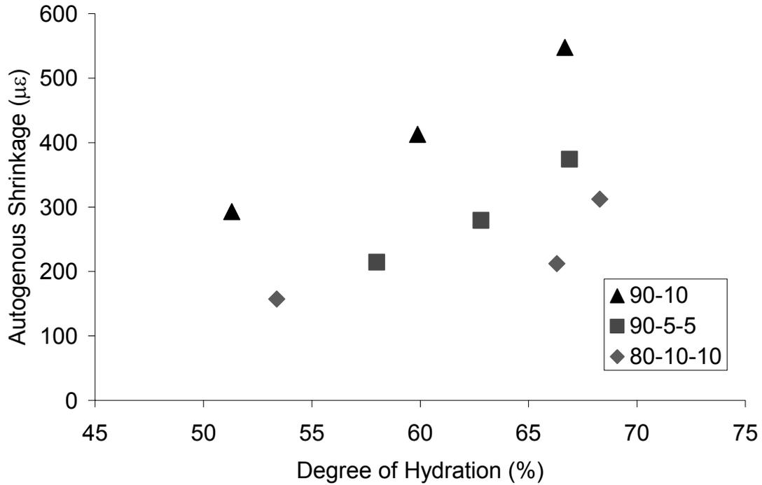
Fig. 1. Relation between the autogenous shrinkage and the degree of hydration
