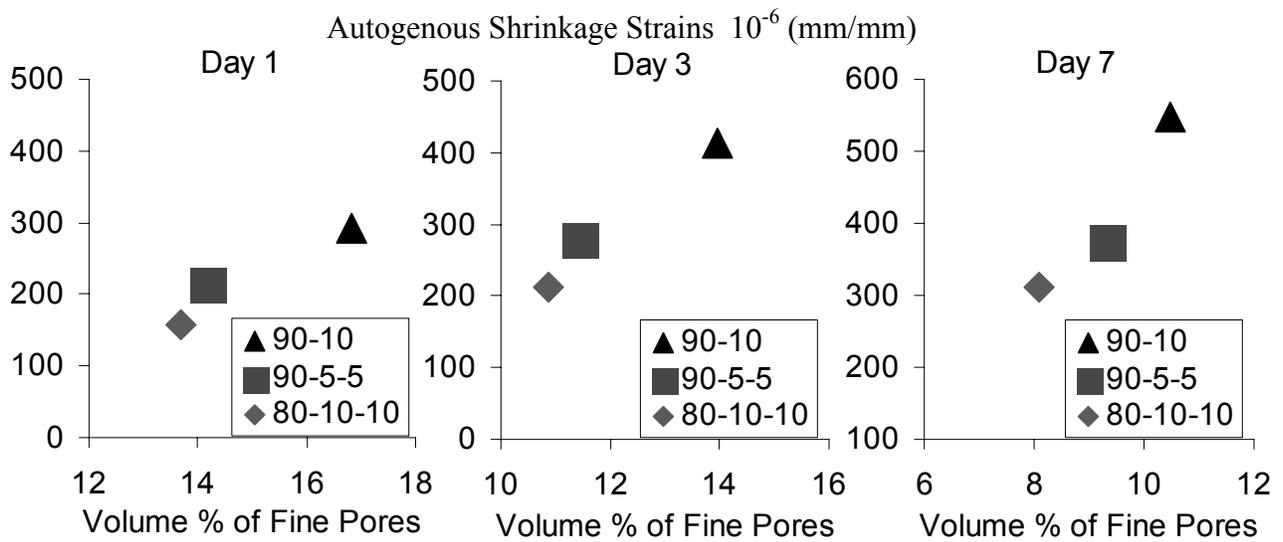
Fig. 2. Relation between the autogenous shrinkage and the volume of finer capillaries (of radius smaller than the critical pore diameter).
