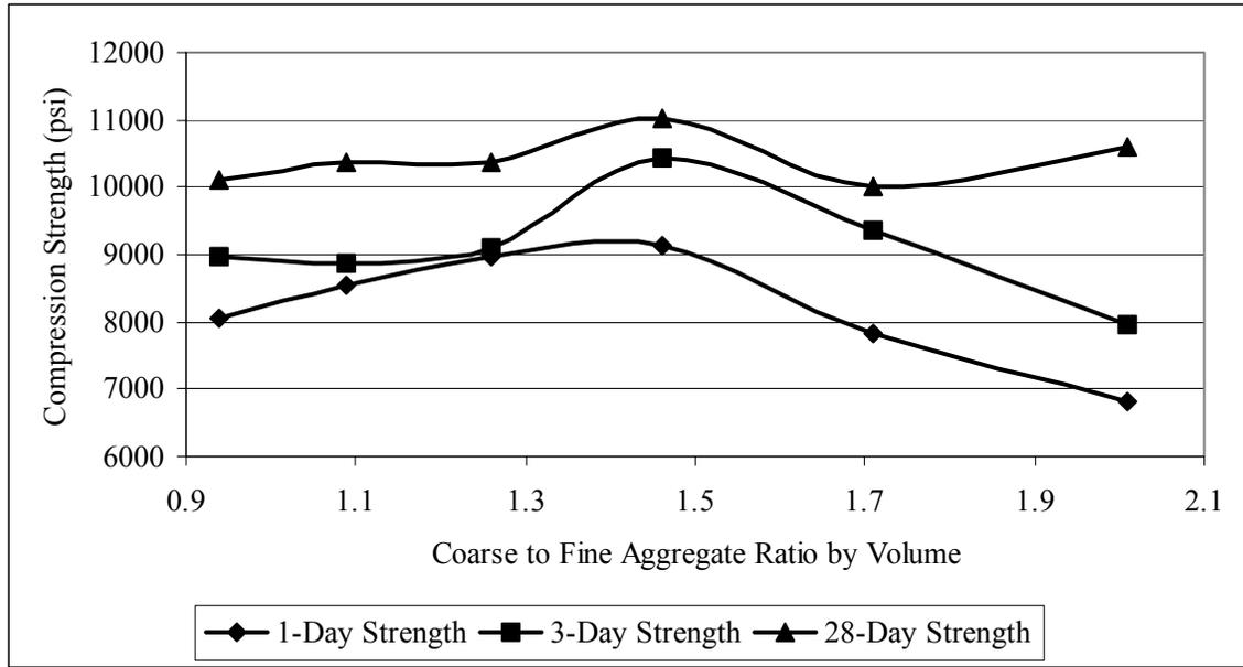
Figure 4. Results of Varying Coarse to Fine Aggregate Ratio
