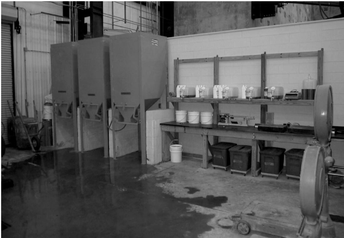
Figure 1. Aggregate Hoppers and Cement / Admixture Proportioning Station
