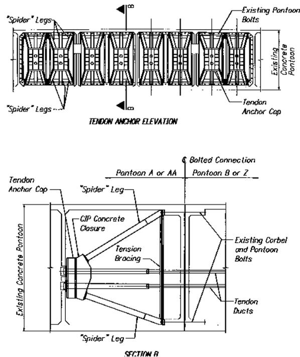
Fig. 2 The top sketch is a full width section of the bridge at the tendon anchor location. The section below shows the “spider” anchor.
