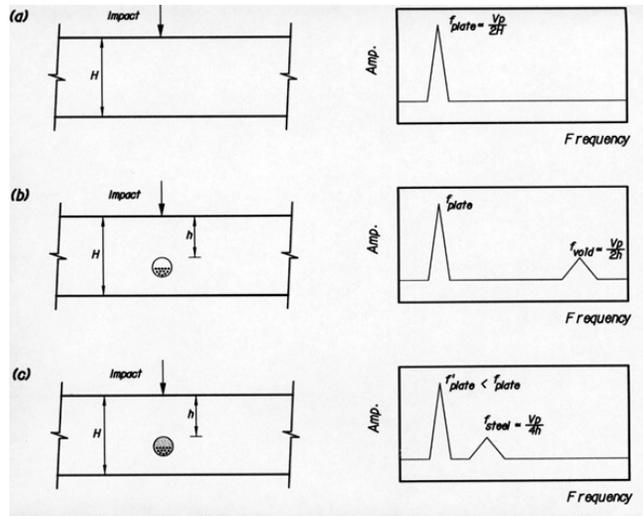
Figure 9 - Basic impact-echo for a plate containing post-tensioning ducts (a) solid plate, (b) duct containing a void, and (c) grouted duct.
