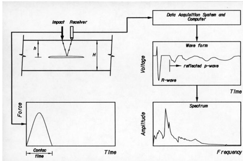
Figure 8 - Diagram of the Impact-Echo method
