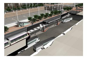
Fig. 3 – Rendered split section of Second Street showing LRT at street level with transit center on lower level.
