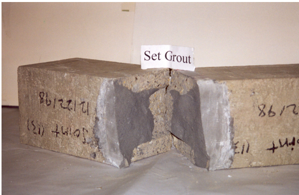
Fig. 7 Failure mode in set grout flexural specimen
