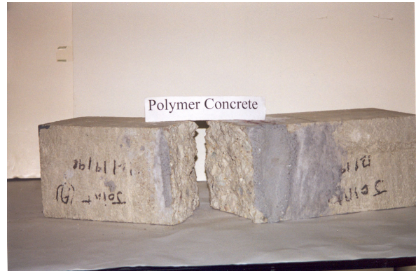
Fig. 8 Failure mode in polymer concrete flexural specimen
