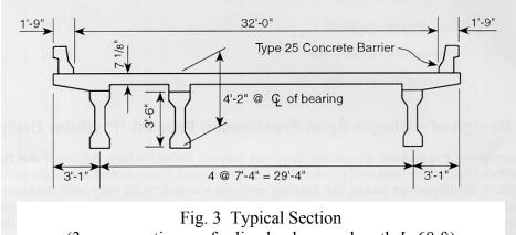
(3-span, continuous for live loads; span length L, 68 ft)
