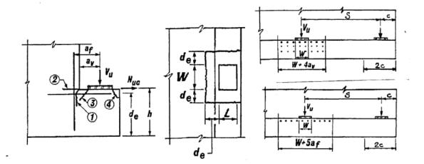
Fig. 5 Notation for Beam Ledges, from AASHTO 5.13.2.5.1,2
