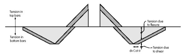
Fig. 4 Variation of Force in Longitudinal Steel of 2-Span Pre-cast Girder Bridge with an Inverted-T Bent Cap (Notes to Fig. 4: 1. Dapped ends at the bent cap mean that girders are indirectly supported, and that shear demand in longitudinal steel must be considered at the center support, as shown above. 2. Not to scale. 3. Enveloping of tension due to maximum positive and maximum negative flexure is not shown. In other words, the
