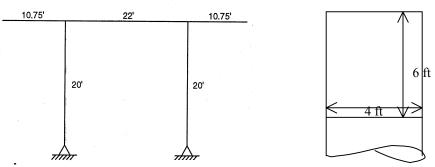
Fig. 2 Bent Cap Elevation and Section
