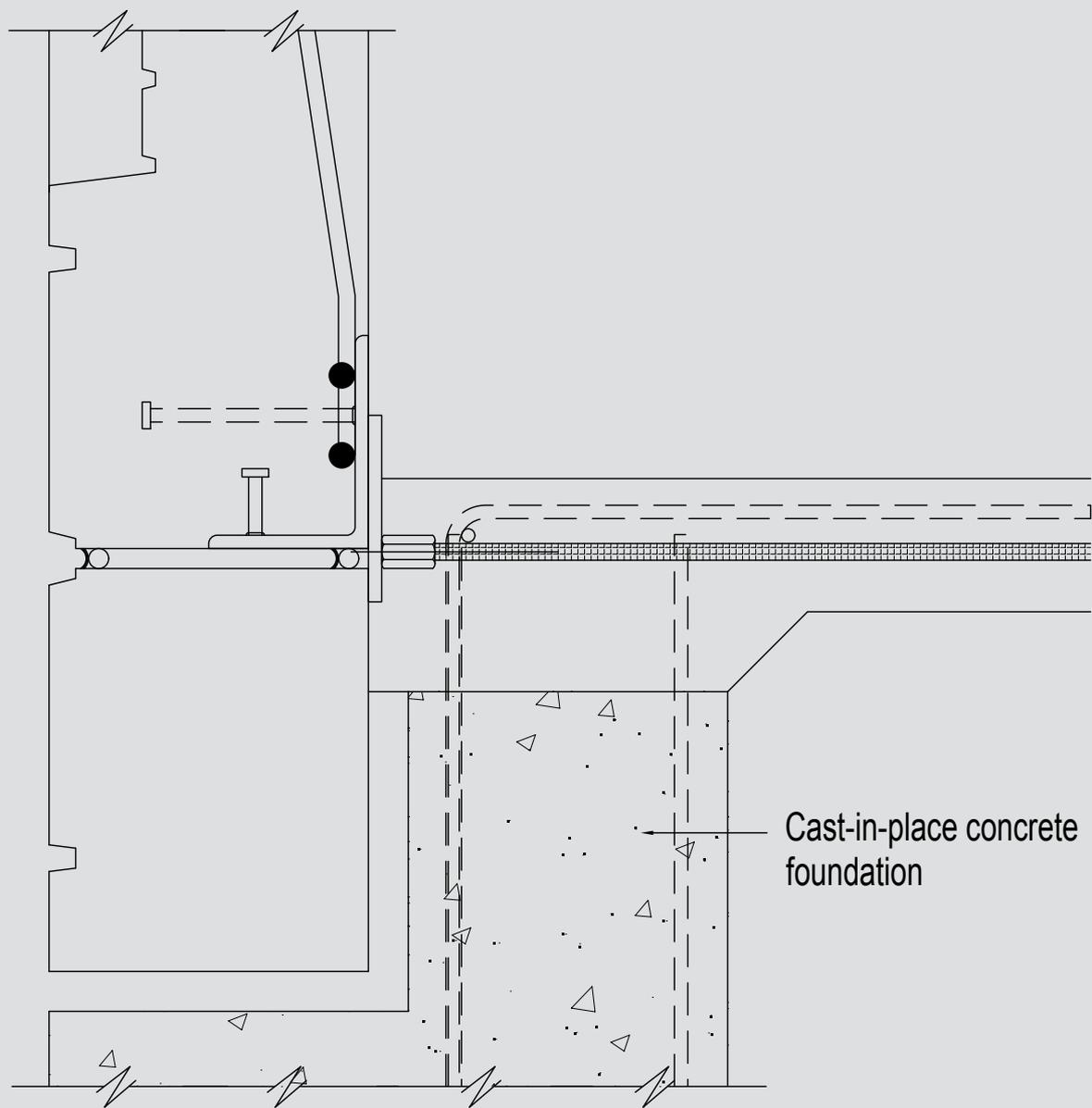
**Figure 6.** Panel-to-structure shear connection at base.
