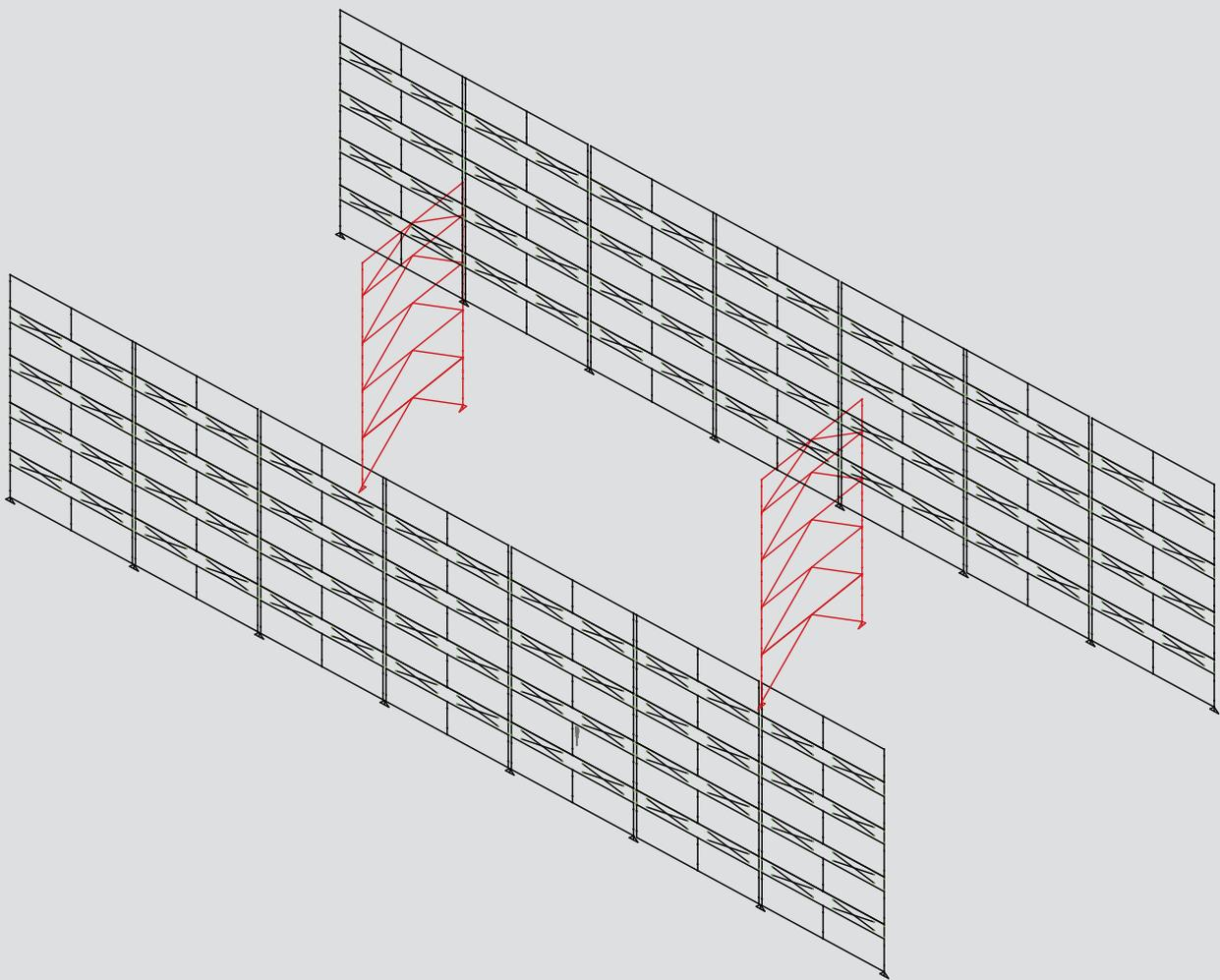
**Figure 3.** Three-dimensional view of numerical model of one of the buildings. Precast concrete panels are shown at the perimeter and internal steel K-braces are used for lateral resistance in the perpendicular axis.
