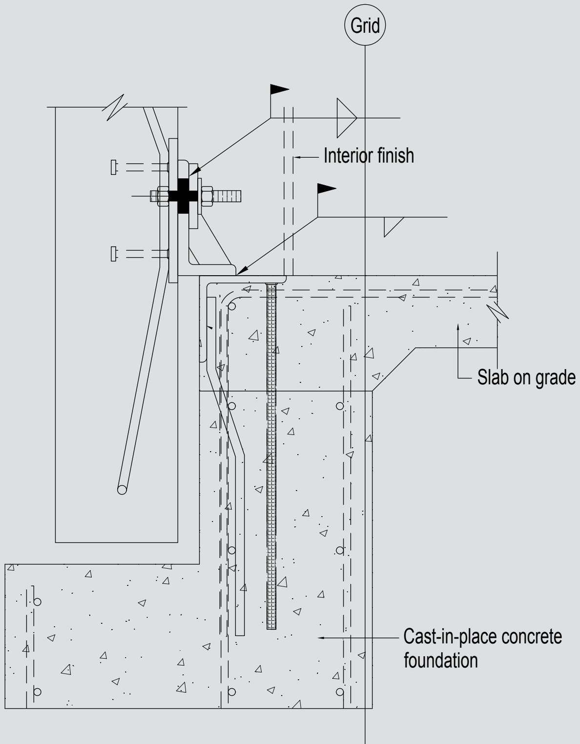
**Figure 7.** Panel-to-structure tension connection at base.
