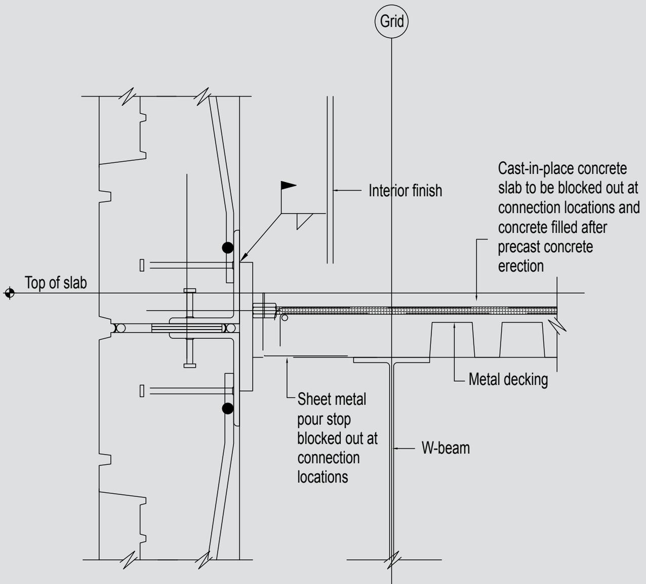
**Figure 5.** Section depicting the in-plane horizontal-shear-resisting connection.
