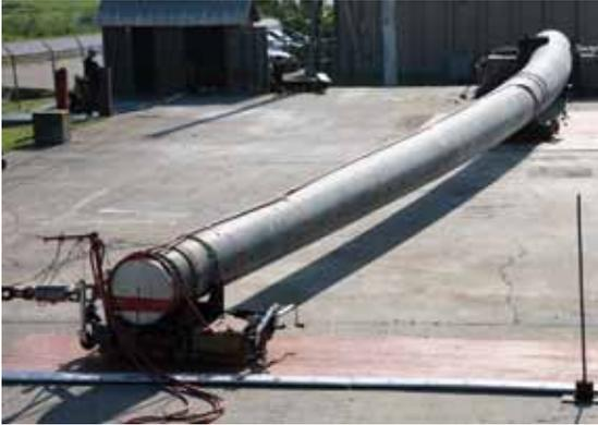
Horizontal deflection test of 115 ft (35 m) spun concrete pole. Once the load was removed, the pole returned to its original shape and the cracks closed. The pole was later installed. Photo by Fouad H. Fouad.
