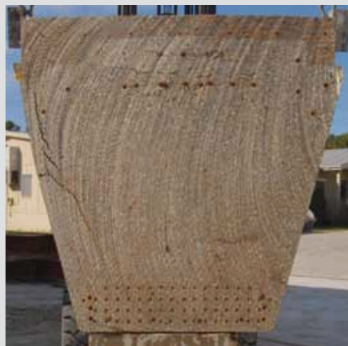
Severe cracking parallel to the surface
