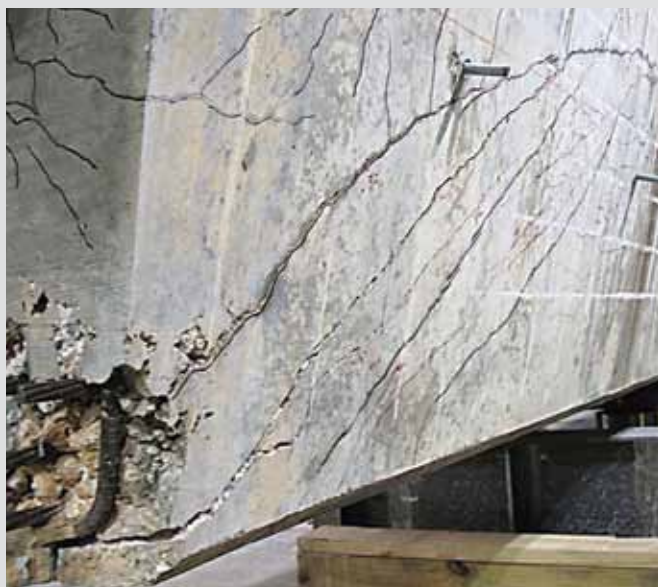
Cracking in the transfer length
