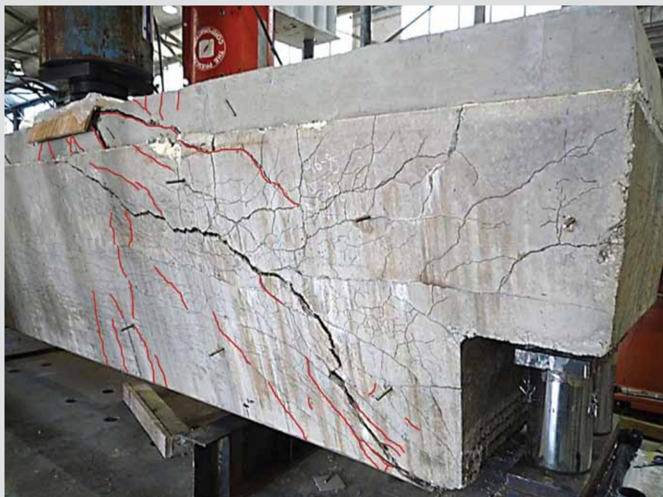
Postfailure widening and extension of alkali-silica reaction and delayed ettringite–formation cracks
