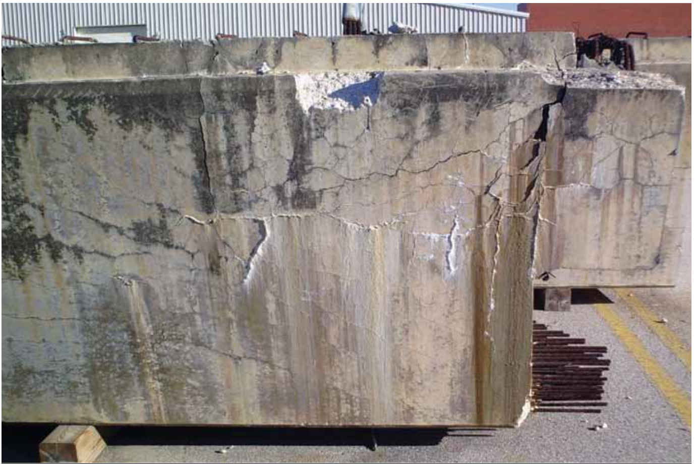
Figure 3. Visual effects of alkali-silica reaction and delayed ettringite formation.
