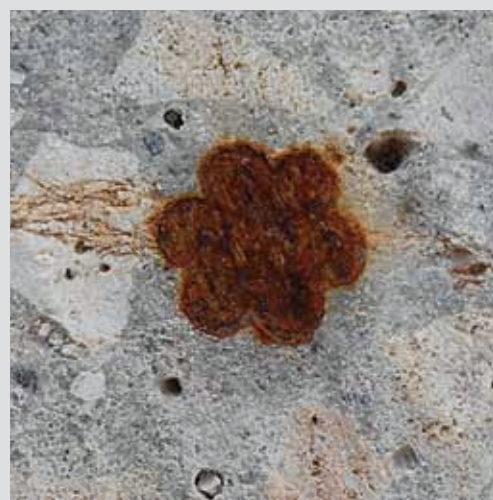
Fine horizontal interstrand cracking
