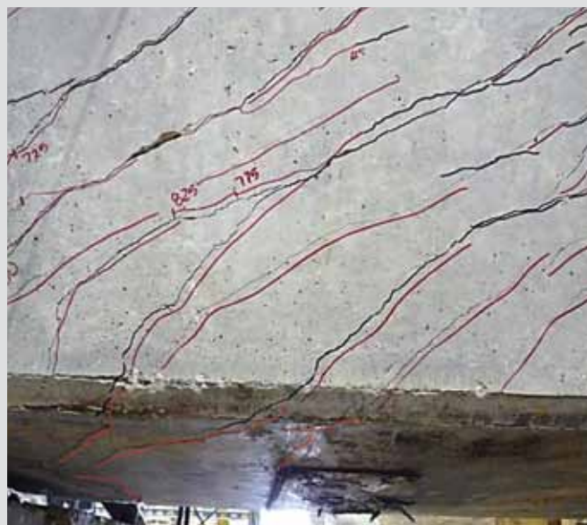
Bottom-side anchorage cracks
