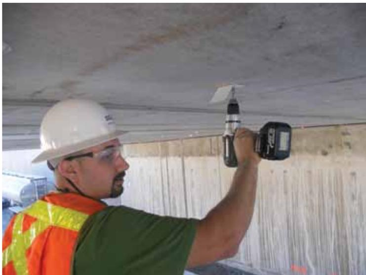
Juliano installs a reflective target for monitoring deflections on the Pembroke Bridge. The target is at a 45-degree angle to the laser beam. **Photo courtesy of Applied Geomechanics.**
