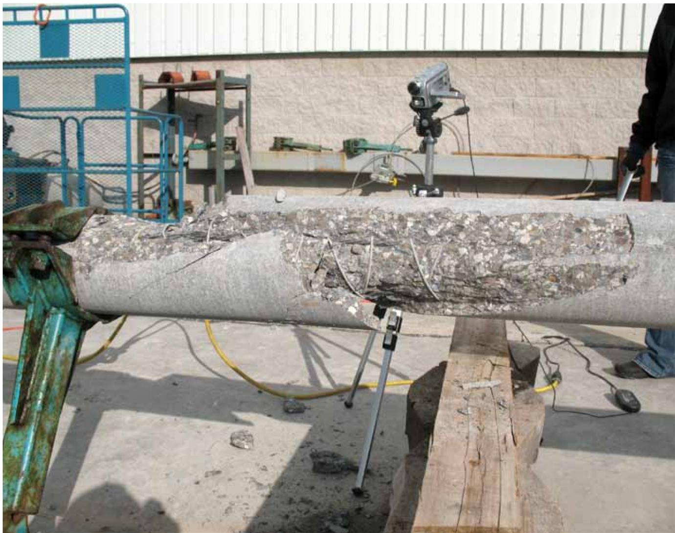
**Figure 6.** Typical loading collar failure.
