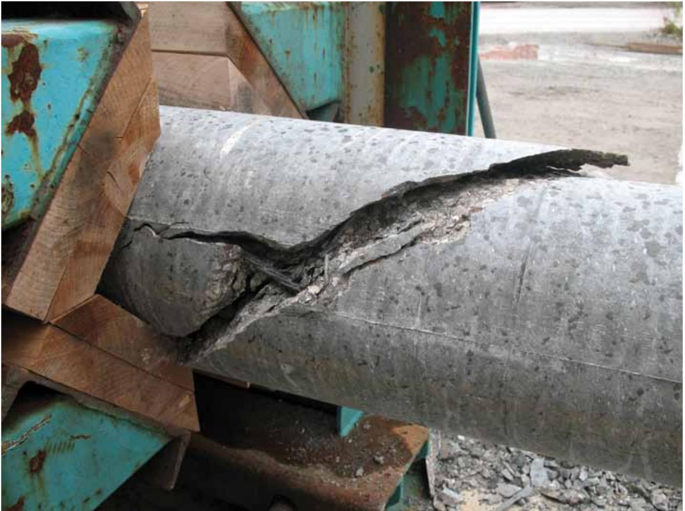
**Figure 7.** Typical butt clamp failure.
