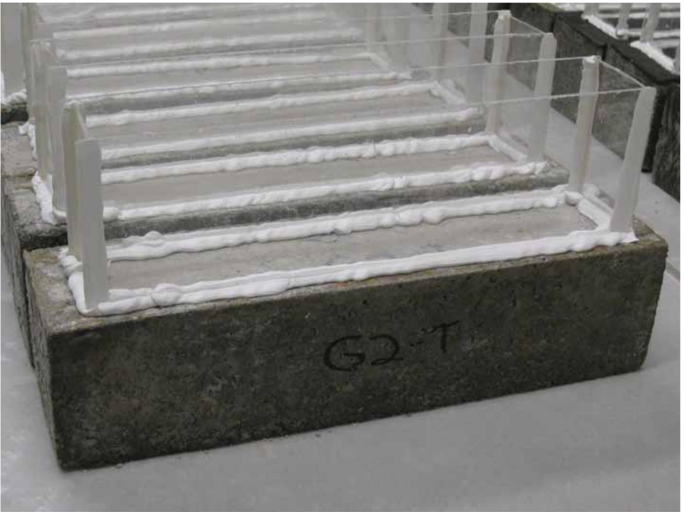
**Figure 10.** Specimens with water dams.
