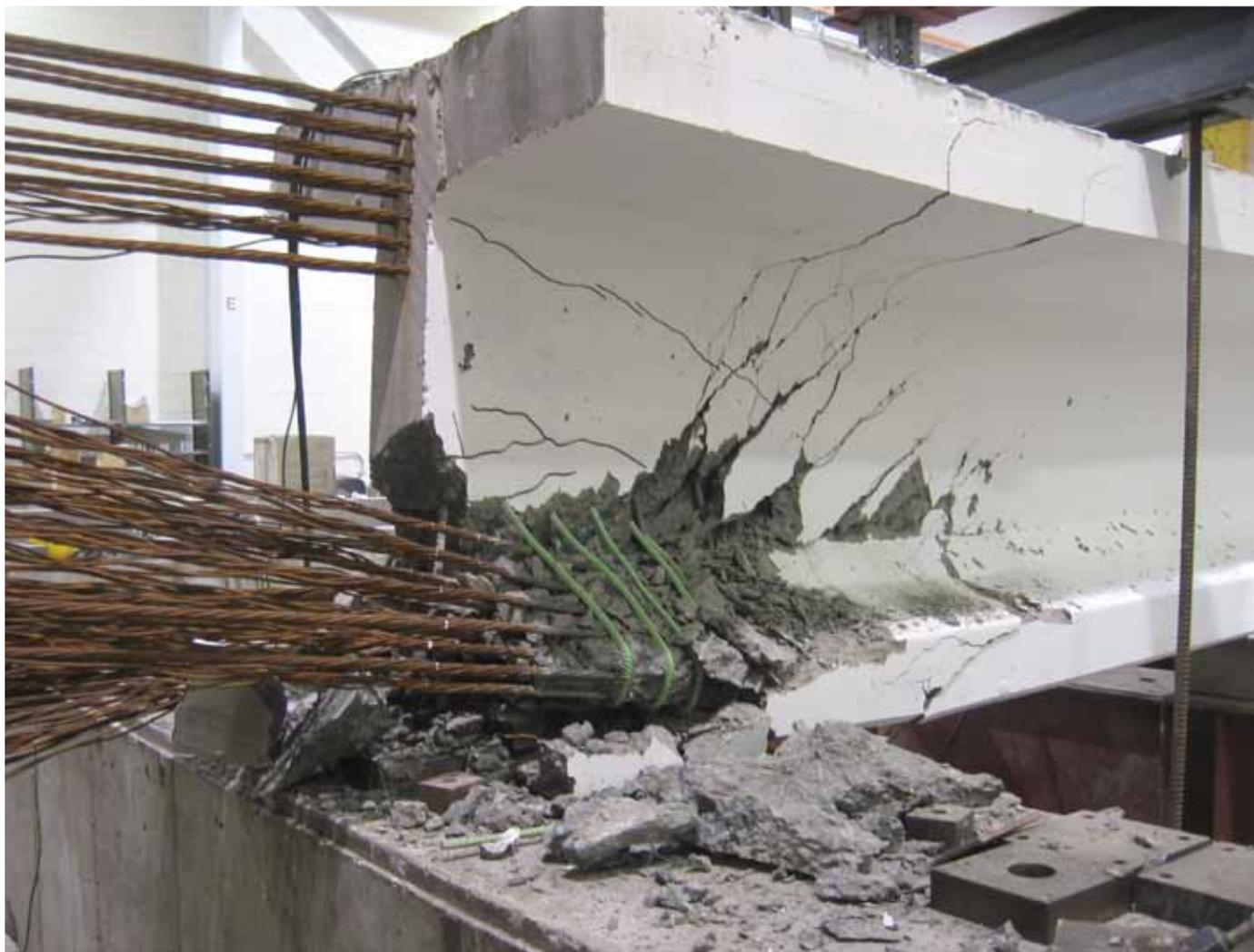
**Figure 7.** Premature failure of end VA1R due to inadequate bearing area.
