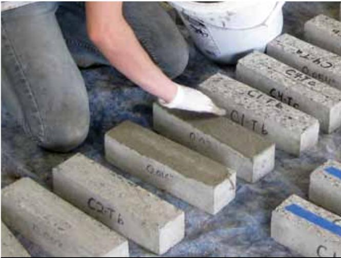
**Figure 9.** Hand application of the hydraulic cementitious material.
