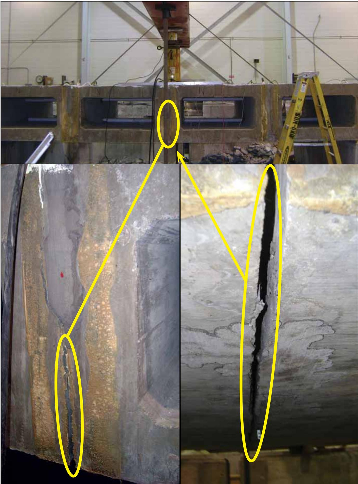
**Figure 12.** Side and underside cracking.
