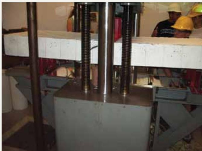
**Figure 3.** Tests were conducted in simple bending with full-width supports at ends of precast concrete slab and full-width loading at center span.
