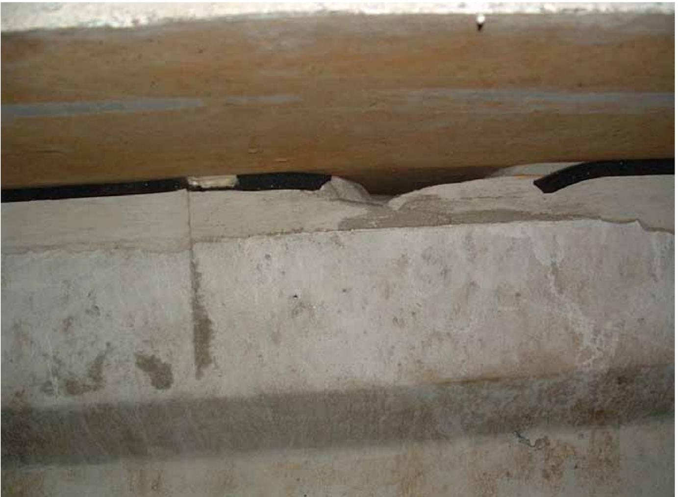
**Figure 9.** Void in grout between haunch and panel. This void was near the midspan of the specimen, where shear was low, and was not detrimental to the performance of the shear connection.
