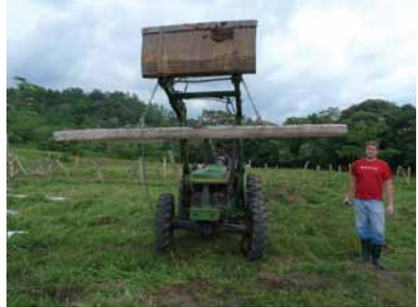
The precast concrete lifting system is tested for use in the construction of an Engineers Without Borders bridge in Canchias, Honduras. Courtesy of Dale Thomas of CH2MHill.
