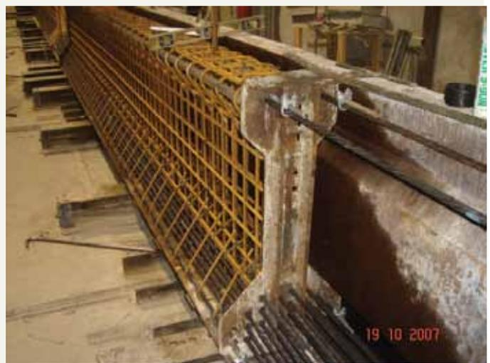
**Figure 5.** Auxiliary reinforcement of the tested girders.
