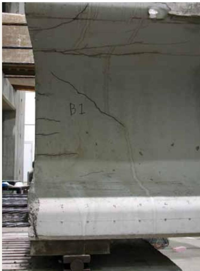
**Figure 7.** End-zone cracking in girder A.
