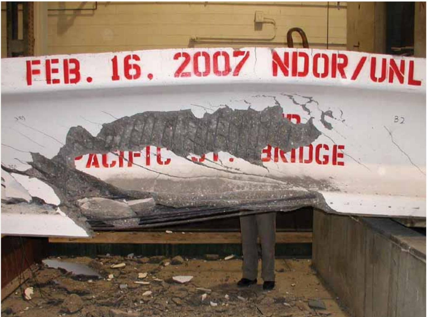
**Figure 16.** Failure of girder A.
