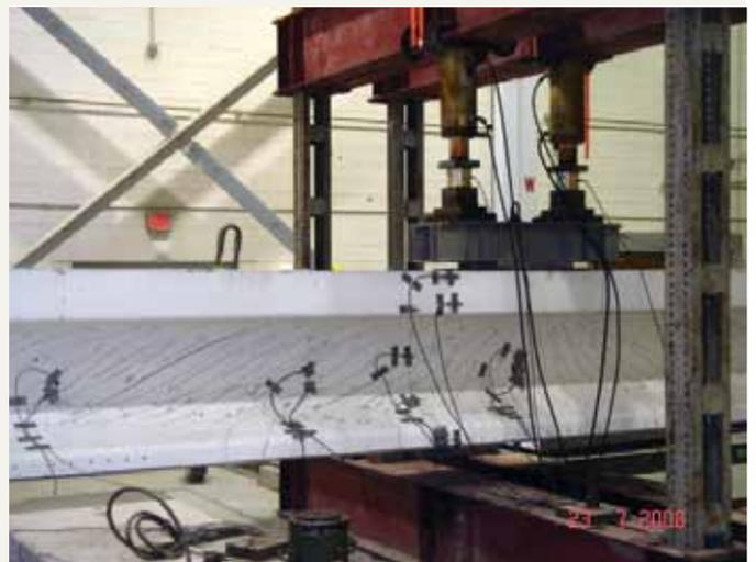
**Figure 17.** Cracking of girder B under maximum load.
