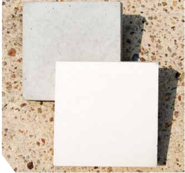
**This white concrete block sample of High Concrete Group's new high-solar-reflectance precast concrete has a solar reflective index of 82. Courtesy of High Concrete Group.**
