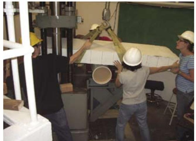
**Fig. 6.** Lowering a precast concrete panel onto rollers for positioning.
