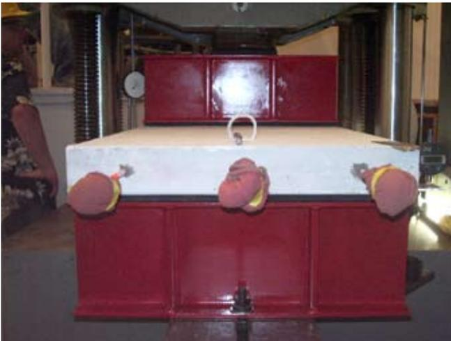
**Fig. 5.** Isometric and end views of overall test setup with the Test 1 precast concrete panel.
