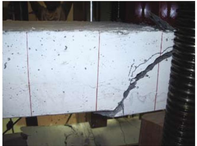
force of 8.15 kip (36.3 kN) (Fig. 11). Predicted maximum force and associated relative displacement were 7.02 kip (31.2 kN) and 1.2 in. (31 mm), respectively (Fig. 11). Predicted displacement capacity was 1.84 in. (46.7 mm) at a compressive strain for the unconfined concrete of 0.005.
