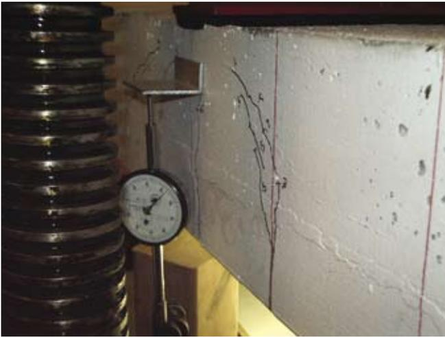
Fig. 13. Displacement target of 0.6 in. (15.2 mm), Test 2.
