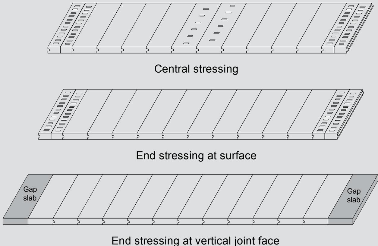
**Figure 7.** Schematic of three precast, prestressed concrete pavement systems.
