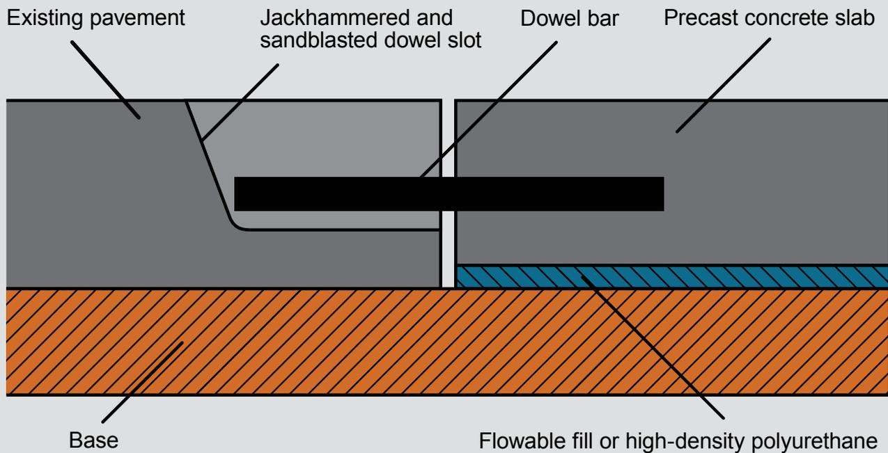
**Figure 1.** Schematic of the intermittent repair application. Source: Data from Hall and Tayabji (2008).
