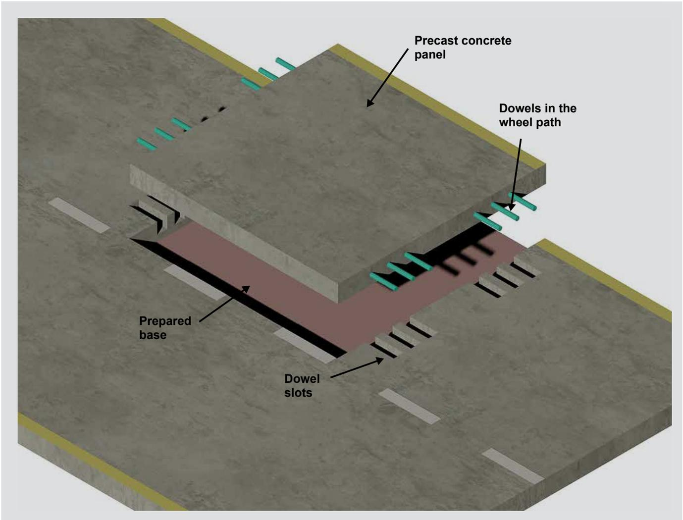
**Figure 2.** One scheme for intermittent repairs.
