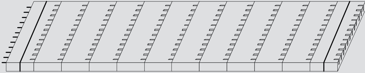
**Figure 9.** Incrementally connected precast concrete pavement.
