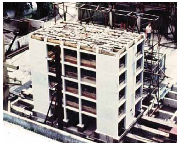
Figure 12. Five-story precast concrete structure (model scale 1:4) during shake table tests.
