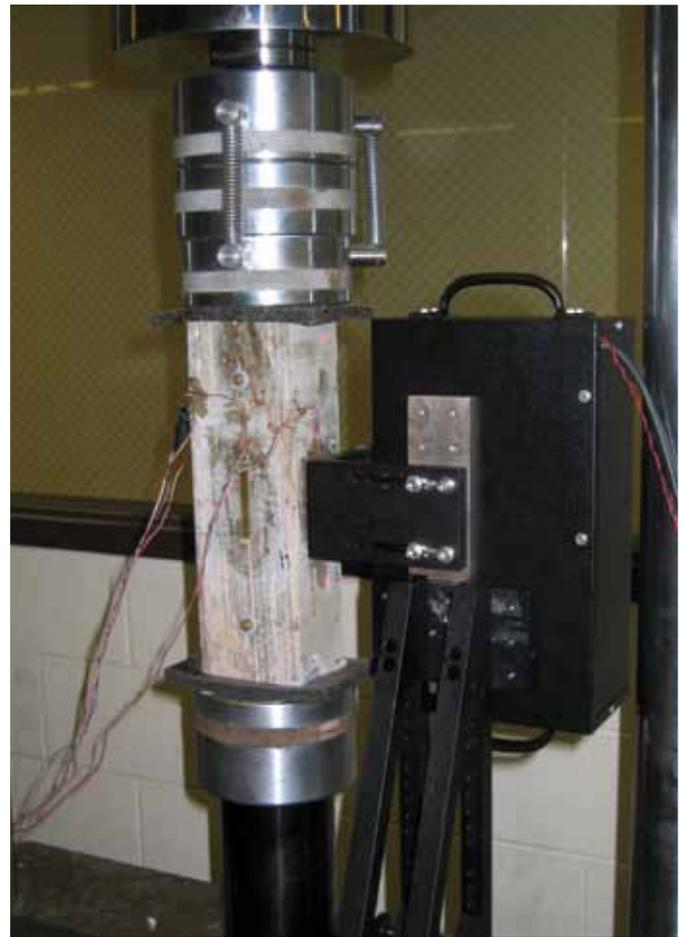
**Figure 5.** Comparison of laser-speckle imaging method with electrical resistance strain gauges on concrete prism in a universal testing machine.
