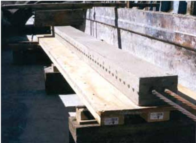
**Figure 1.** A small pretensioned concrete member was used to measure the transfer length.
