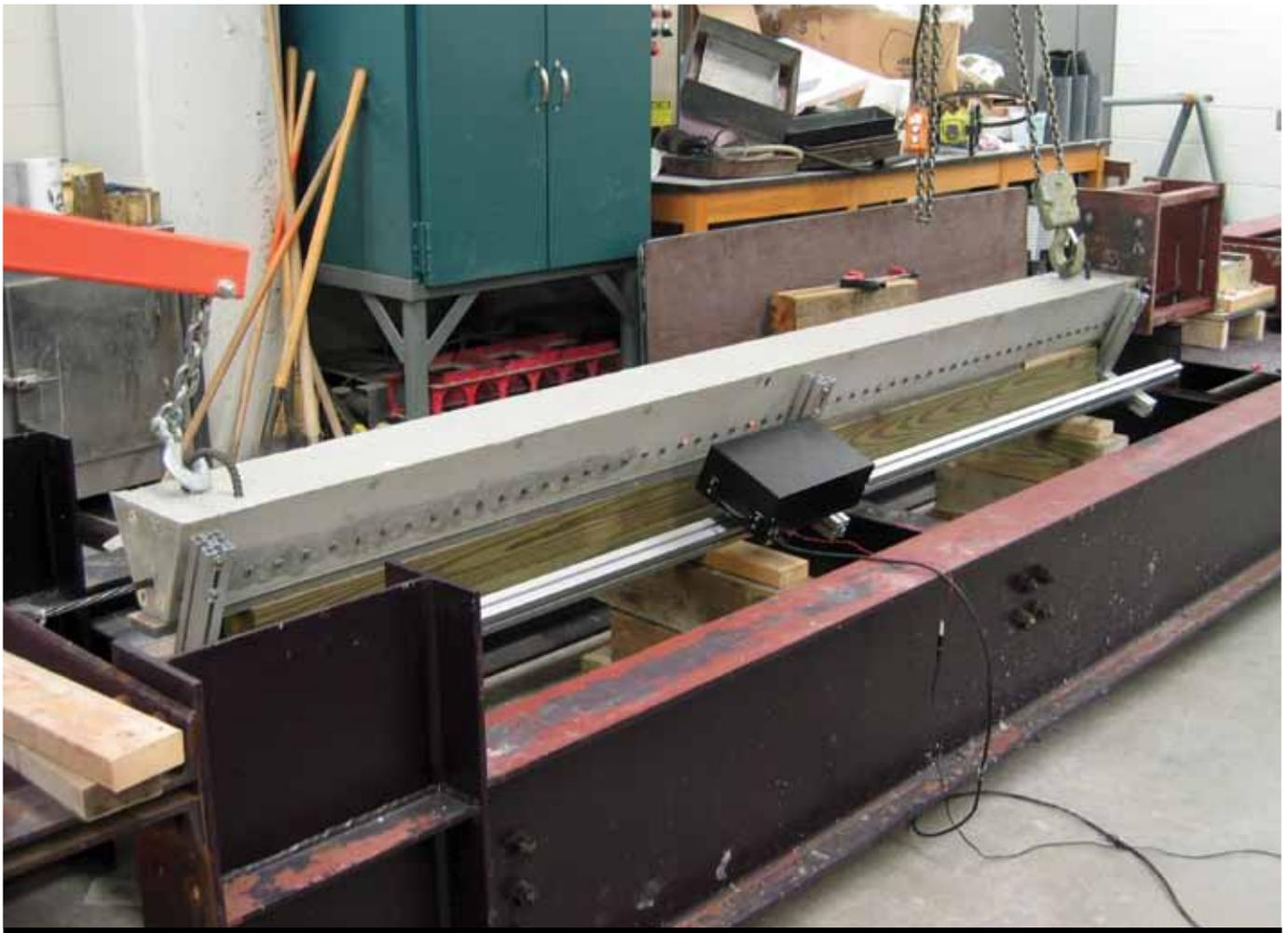
**Figure 7.** The measurement of surface strains was accomplished using both the traditional surface-mounted method and the noncontact laser-speckle imaging method.
