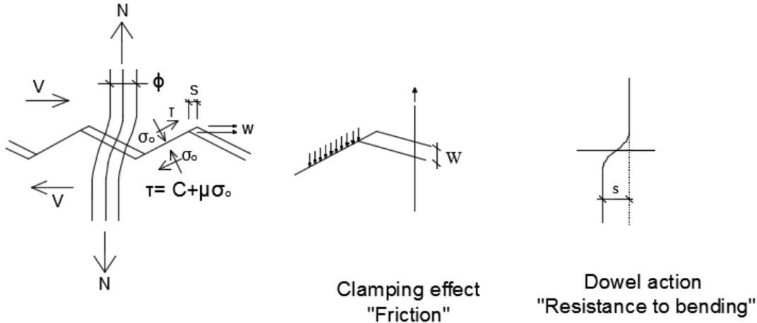
Figure 2: Interface shear resistance mechanism (Randi, 1997)
