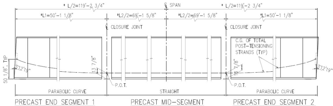
Fig. 5 Post-tensioning Profile (Note: 1 in. = 25.4 mm; 1 ft = 12 in.)
