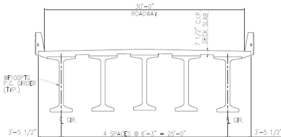
Fig. 3 Chief Joseph Dam Bridge Typical Section (Note: 1 in. = 25.4 mm; 1 ft = 12 in.)
