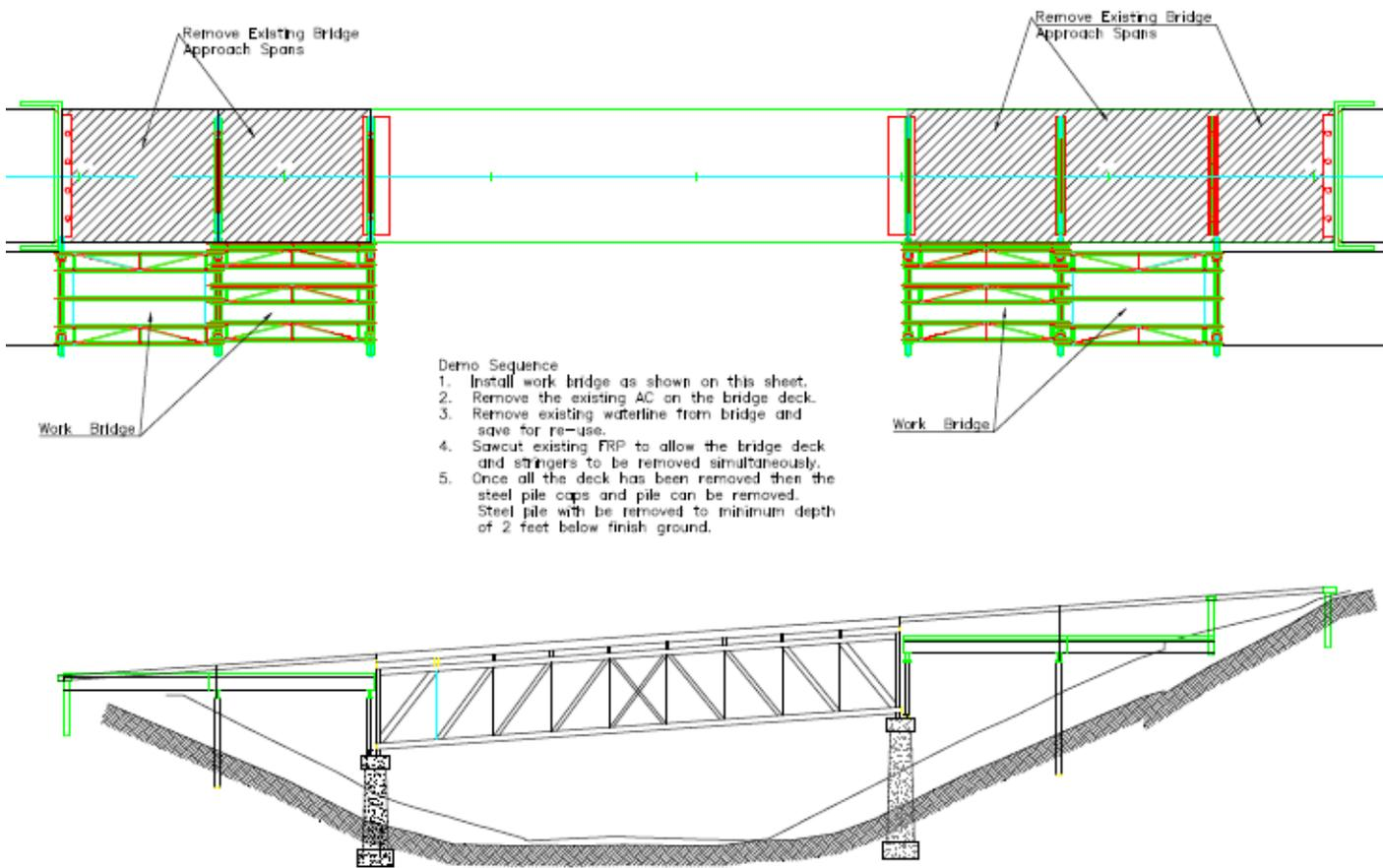
Fig. 7 Bridge Construction Sequence – Stage 1
