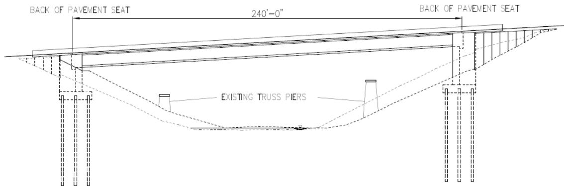
Fig. 2 Chief Joseph Dam Bridge Elevation View (Note: 1 in. = 25.4 mm; 1 ft = 12 in.)
