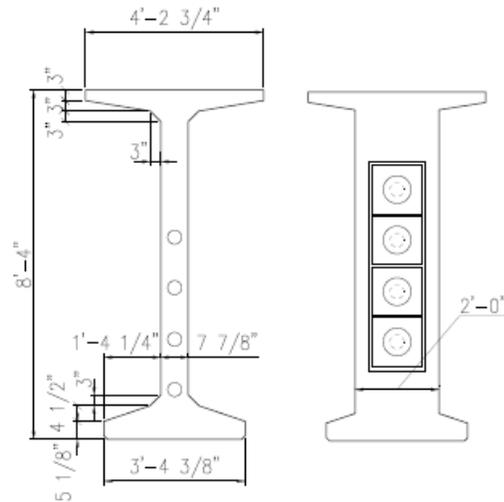
Fig. 4 Girder Section (Note: 1 in. = 25.4 mm; 1 ft = 12 in.)
