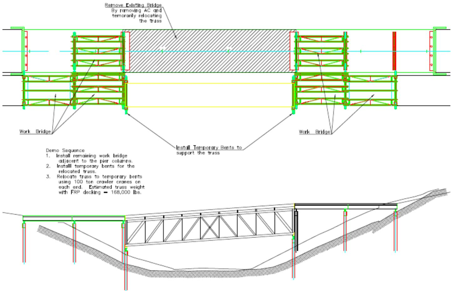
Fig. 7 Bridge Construction Sequence – Stage 2
