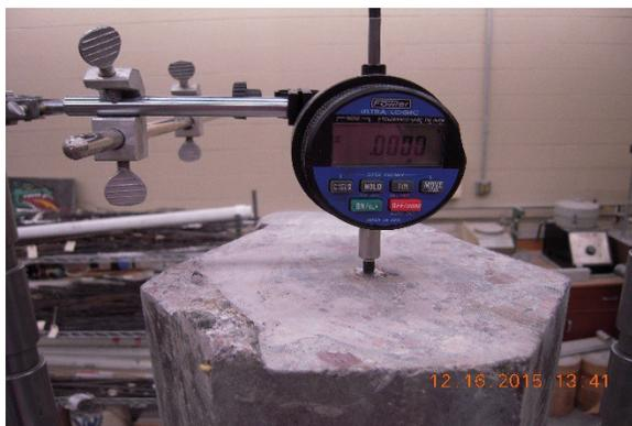
Fig. 7 Placement of dial gage on center wire of strand
