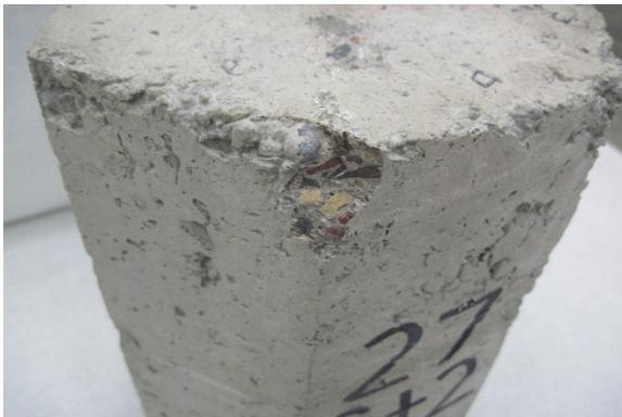
Fig. 16 Specimen 27St2 crushing on live end
