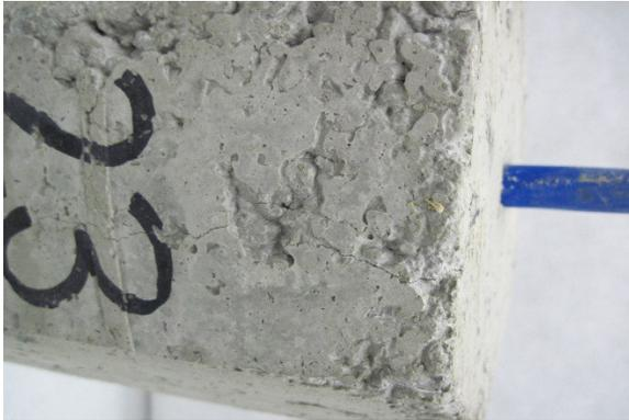
Fig. 15 Specimen 23St2 small cracks
