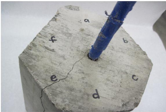
Fig. 12 Specimen 7Sp2 cracking on live end
