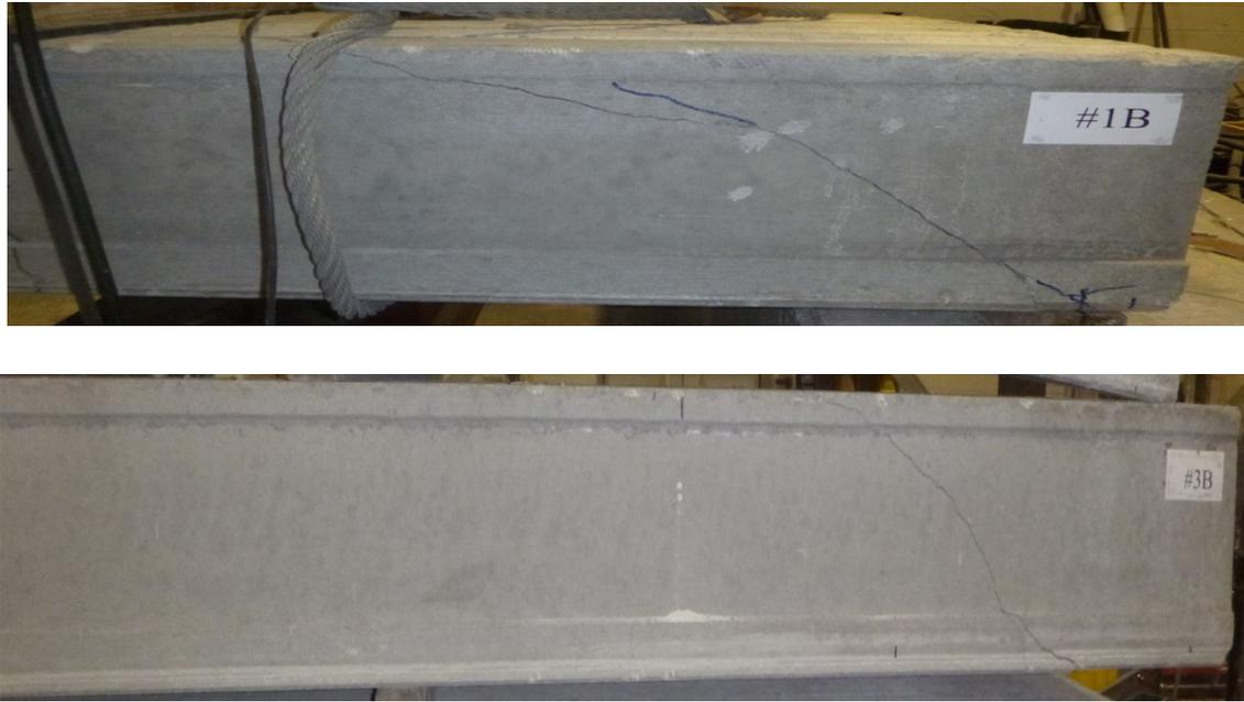
Figure 7: Web-shear failure cracks
