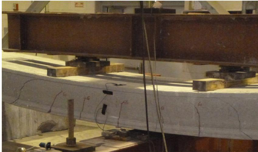
Figure 9: Flexure cracks under cracking load
