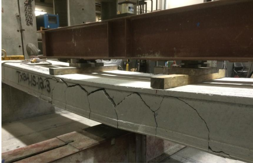
Figure 10: Flexure-shear cracks under ultimate load
