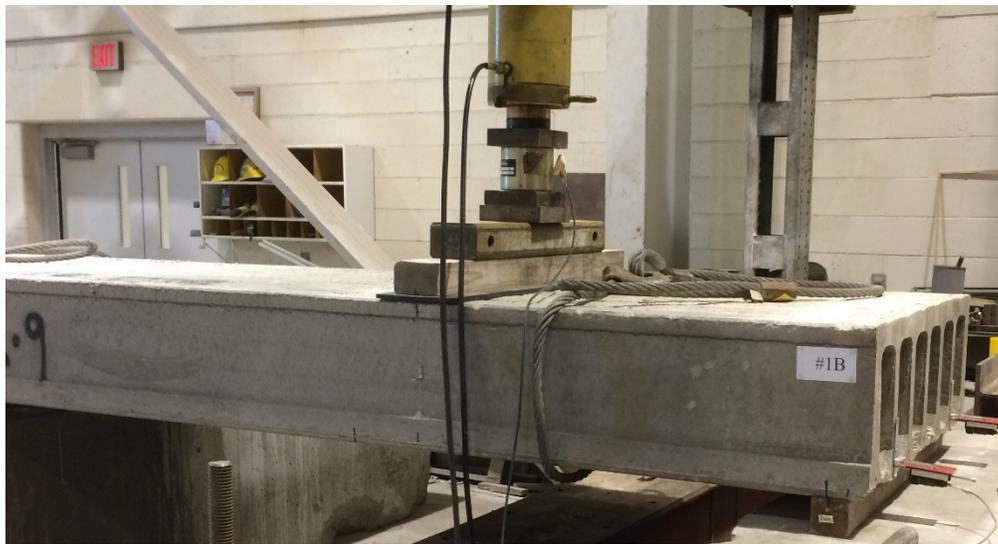
Figure 3: Web-shear test specimen supported by 48 in long 4x4 dimension lumber
