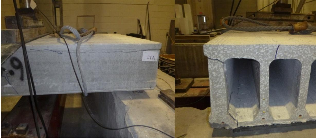
Figure 5: Failure of specimen #1A due to inadequate bearing
