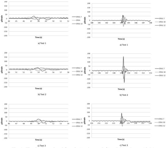
Fig. 16 First load test: Load Case 2, 5 mph pass (left) and 45 mph pass (right)
