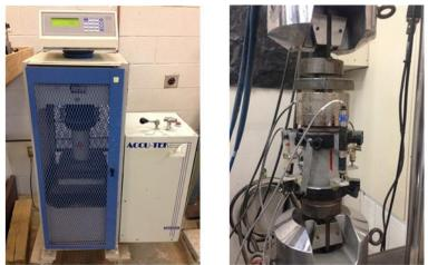
Fig. 7 Compressive strength testing (left); modulus of elasticity testing (right)
