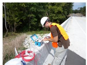
Fig. 8 Strain readings recorded with Vishay P3 strain indicator
