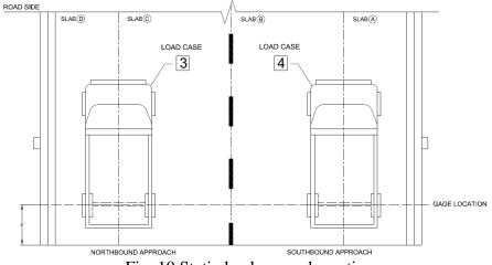
Fig. 10 Static load case schematic
