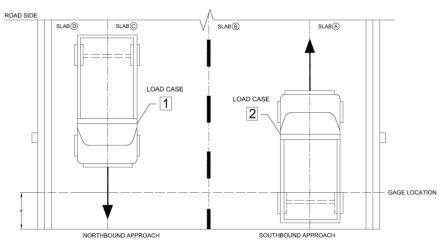
Fig. 9 Dynamic load case schematic
