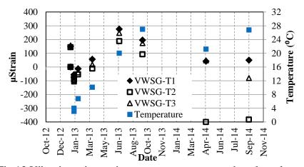
Fig.13 Vibrating wire strain gage measurements - shear key closures
