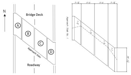
Fig. 1 Layout of precast approach slab system
