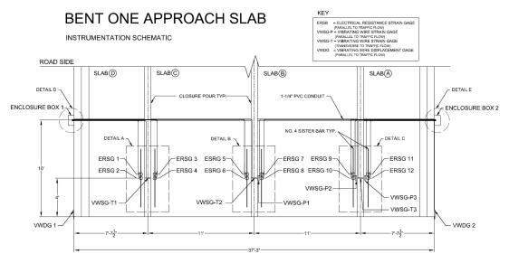
Fig. 5 Bent One approach slab schematic - plan view
