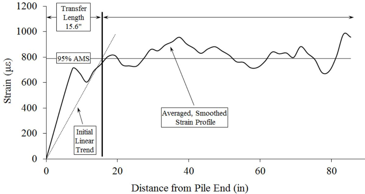
Fig. 6. Transfer length plot for pile SS 2205 #1 – North End, 14 days after prestressing.
