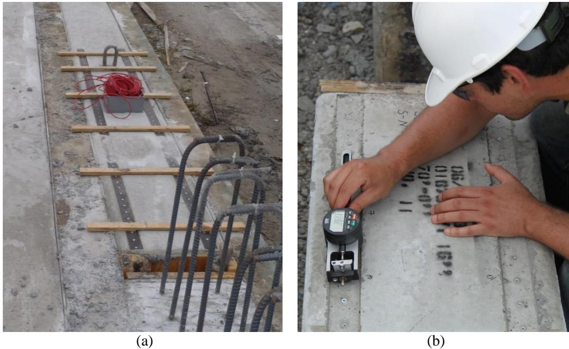
Fig. 5. (a) Embedded elements left uniformly spaced points to be measured with a DEMEC gauge, (b) Measurement of deformations at the surface of the piles. 86 measurements were made at each pile end.
