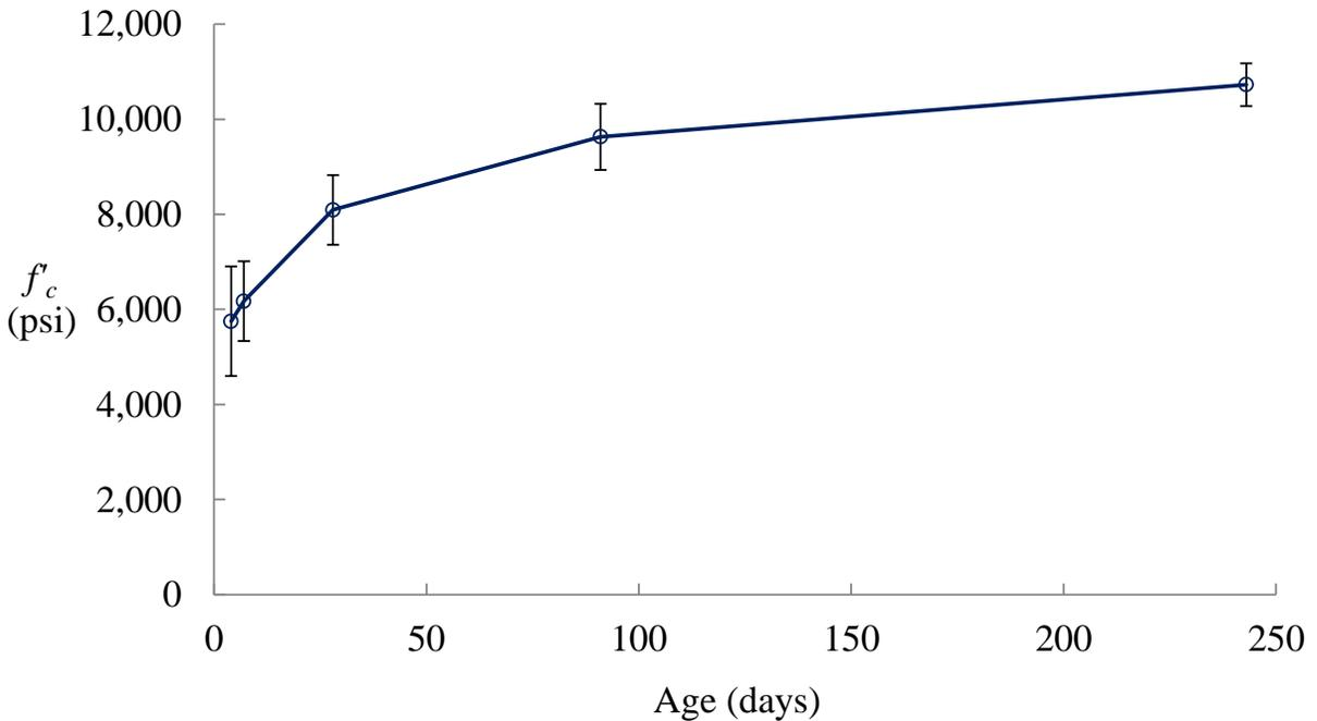
Fig. 3. Average concrete compressive strength at 4, 7, 28, 91, and 243 days. Error bars show standard deviation.
