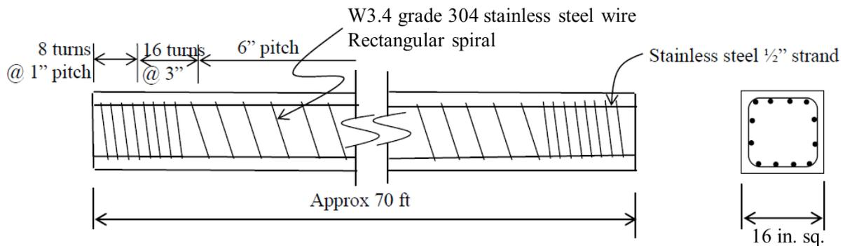
Fig. 1. Typical 2205 stainless steel test pile.
