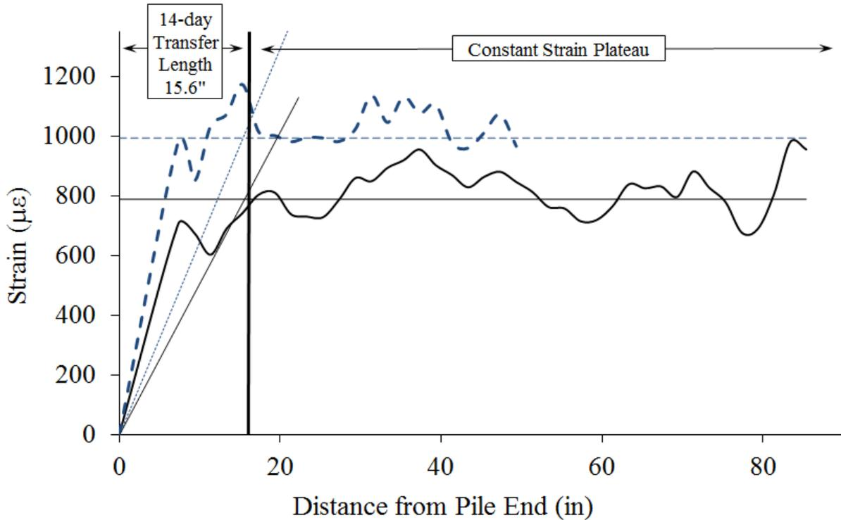
Fig. 7. Comparison of transfer length calculation for pile SS 2205 #1 – North End, after 14 days (black line) and after driving process (day 273, dashed blue line).
